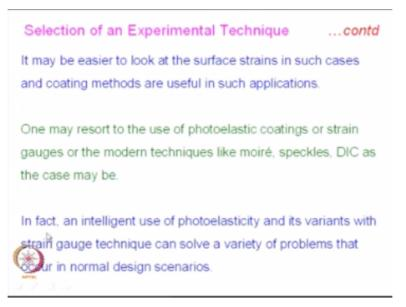
It may be easier to look at the surface strains in such cases and coating methods are useful in such applications. One may resort to the use of photo elastic coatings or strain gauges or the modern techniques like Moire speckles, digital image correlation as the case may be. In fact, an
