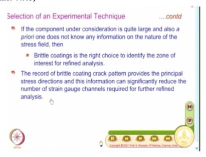
So, look for whether this could be employed for your problem on hand. On the other hand, if the component under consideration is quite large and also a priori one does not know any information on the nature of the stress field, then combine brittle coatings, identify iron strain gauges, so use brittle coatings to identify zones of interest for refined analysis, continue the refined analysis based on strain gauges.
