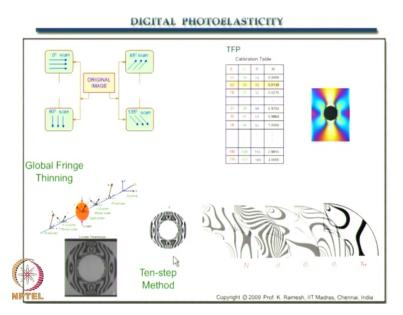
Then we moved on to another aspect of photoelasticity which is becoming very popular these days known as digital photoelasticity. An initial stage they had developed algorithms to thin the fringes that is what you have as the global fringe thinning algorithm. So it employed scan at 0 degree, 45 degree, 90 degree and 135 degree. And logical operators were used to get this skeleton free of noise.
