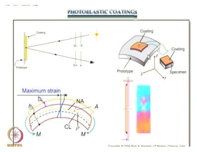
And we said, we also need to have methodologies to analysis prototypes that was discussed in photoelastic coatings. And I said all the coating techniques share a commonality, we have photoelastic coatings, we have brittle coating, and to an extent, you can also think of strain gauge as a coating applied on the material. And one of the key concept here is the strain in the prototype is faithfully transferred to the coating.
