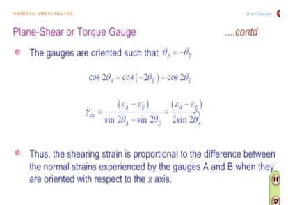
So when I have theta A=- theta B I get gamma xy as epsilon A-epsilon B/2 sin 2 theta A. And you know, in normal strain gauge measurements you connect 1 strain gauge to a Wheatstone
