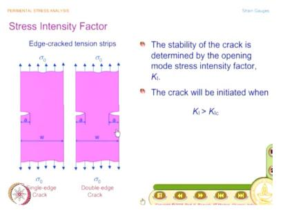
So that is the way I am going to about, but before we going do it, we will also recall what we have learnt in our course on fracture mechanics. What is a stress intensity factor? Essentially the stress field in the vicinity of the crack is possible to write in terms of the stress intensity factor, and you may have multiple cracks in a system, the crack that is critical is going to propagate. And fracture mechanics says that when K1>the fraction toughness that is K1c the crack will be initiated.
