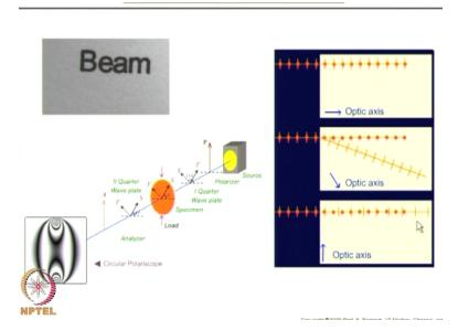
We started with transmission photoelasticity, I said the key concept was when you have model that is loaded, it behaves like a crystal, when it is loaded when the loads are removed it behaves like a normal material. And crystal exhibits a property of birefringence, and this is exploited in photoelasticity, and you are able to view fringe patterns in different optical arrangements, here you have a circular polariscope, you have both the dark field as well as bright field possible.
