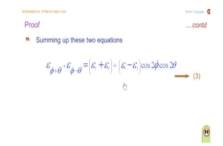
But you will also find out whether you could use a simple normal strain gauge for stress measurement. And when I add these 2 strain quantities, I get this as epsilon 1+epsilon 2 + epsilon1-epsilon 2 multiplied by cos 2 phi\*cos 2 theta, and I will further simplify. My focus is finally to get the addition of these 2 strains proportional to a single stress component that is what I am going to show, and we will not evaluate the angle theta.
