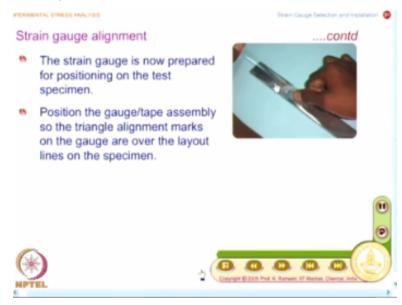
The strain gauge is now prepared for positioning on the test specimen, so you hold it like this and then position it, you position the gauge tape assembly, so the triangle alignment marks on the gauge or over the layer out lines on the specimen. So, you ensured that, you can do this back and forth until you are satisfied that the; whatever the marks on the gauge pattern matches with the layout lines.
