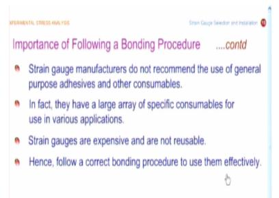
So, the very fact, a professional society conducts an examination and makes that the certificate is valid for a period of 3 years shows how important the strain gauge bonding is and if you look at the strain gauge manufacturers, they do not recommend the use of general purpose adhesives and other consumables. For strain gauge instrumentation, you should go in for specific adhesives and other consumables like a cellophane tape, we will see later.
