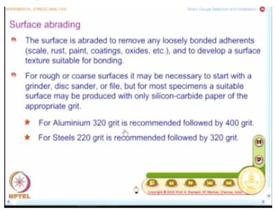
So, you need to keep using new sponges until the cotton gauze is white, so use consumables liberally, so now you have removed the grease, the next step is surface abrading and why do you do this? The surface is abraded to remove any loosely bonded adherents and to develop a surface
