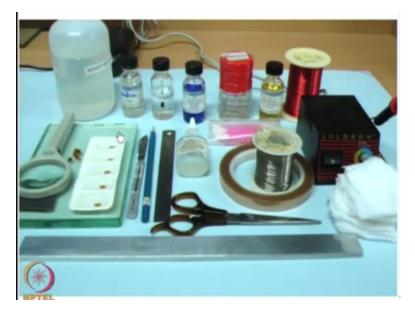
It is not that you go, quickly take the adhesive and then quickly go and do the same gauge bonding, you do not do it like, you have to follow a procedure you have to be systematic. The reason is; you are measuring very small quantities and perfect bonding is a must, it is not a trivial step and this shows, what is the strain installation kit; you have a verity of fluids for cleaning, for catalyses, for adhesives.
