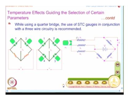
So, the advantage is; there is you maximise the signal 4 times and also has intrinsic temperature compensation but we have seen in many applications where you are interested in strain measurement, you may end up using only a quarter bridges. So, how do I do, when I have quarter bridge arrangements? We have seen how to minimise the error, when we use a quarter bridges instead of 2 wires circuitry, go for a 3 wire circuitry.
