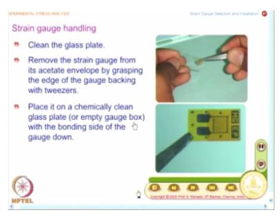
You cannot cut short steps, if you cut short steps you are not guaranteed with proper behaviour of the strain gauge system. Now, the surface is prepared, we have to take out the strain gauge and also have a via media, how to align it on the specimen. So, take a glass plate and clean it that is where you are going to keep the strain gauge and you have to remove the strain gauge from its acetate envelope by grasping the edge of the gauge backing with tweezers.
