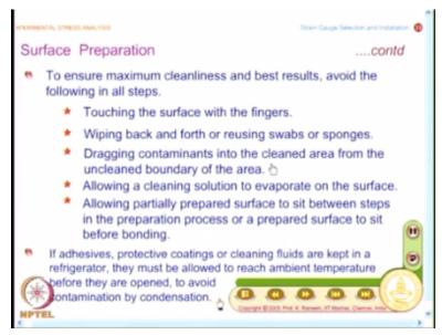
And when you go for plastics or composites, you have to try out the various steps recommended by the manufacturer and follow the recommendation after standardising the procedure. We are only going to look at how to paste a strain gauge on an aluminium surface, it is a very simple one that gives out the various steps and you get an idea, how to go about in general and there are also general recommendations.
