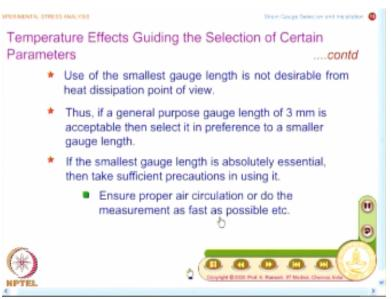
So, if a general purpose gauge length of 3 mm is acceptable, select it in preference to a smaller gauge, so this is a recommendation. So, you need to go in for selecting a longer gauge length from heat dissipation point of view there what you would normally do if you are not exposed to strain gauge technology. On the other hand, if the smallest gauge length is absolutely essential, then take sufficient precautions in using it.
