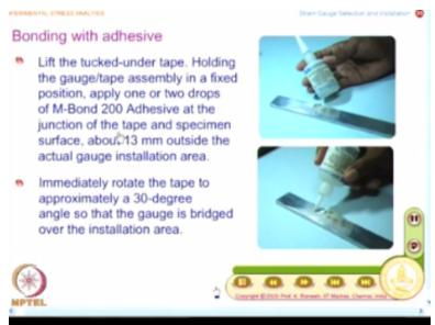
So, you need to read these steps before proceeding, so you need to have a mental picture what way you will have to go about and executed as quickly as possible. So, you have to lift the tucked under tape, holding the gauge tape assembly in a fixed position, apply 1 or 2 drops of M Bond 200 Adhesive, you also have equivalent adhesives at the junction of the tape and specimen surface.
