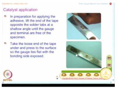
And before we apply the adhesive, we need to apply catalyst. So, you carefully remove this from the surface and that is what you see here, the tape is getting removed and you have to take it and roll it back and fold it and that is what is shown in the next slide.
