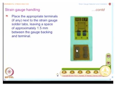
And the focus here is how to simplify your aligning process and in order to simplify your soldering, you also have additional terminals instead of directly using the lead wire up to the strain gauge, you have terminals and you will have a single strand wire connecting the strain
