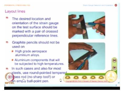
So, these marks have to be aligned at the point of interest for you to align the strain gauge, you need to have layout lines. So, you put a perpendicular line and as I mentioned earlier, you cannot use the graphite pencils on high grade aerospace aluminium alloys or aluminium on components
