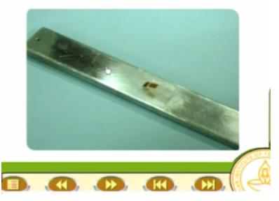
So, what you have here is; you fold it like this, so that easy for you to apply the catalyst and also when you want to put the adhesive, you will you put adhesive at the junction and then press it onto the actual surface and this is what listed here. So, you need to take the loose end of the tape and press to the surface, so the gauge lies flat with the bonding side exposed, you want to take out the tape, fold it like this; fold it like this.
