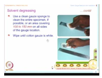
And you need to perform preliminary tests to standardise the process and I said that you should use sufficient the amount of consumables, you should not be stingy in that because your focus is to save the strain gauge, which is expensive and you know, I have this and then I clean it a gauze sponge and you will be surprised to see the surface was looking alright but when I see that gauze sponge, I see that as black.
