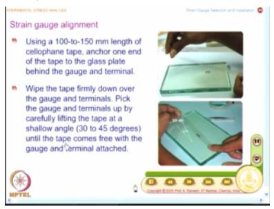
This is just for connecting the strand of wire from the tape to the terminal and in order to align the strain gauge, what you do this; you take a cellophane tape and then paste it on the complete system. So, you have a long cellophane tape taken and even the cellophane tape has to be approved by the strain gauge manufacturer because the adhesive may interfere with the adhesive on the cellophane tape.
