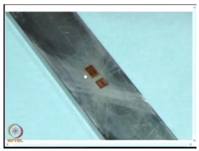
What you see here is; I could see the strain gauge and the terminals aligned on the layout line marks satisfactory, I have a line here and this is aligned with that.
