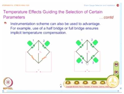
We have also seen that instrumentation scheme can also be used to advantage in handling the temperature effects. So, if you use a half bridge, whatever the temperature changes happen in arm 1, will be cancelled by temperature changes in arm 2, if both the strain gauges are exposed to similar temperature levels and a similar advantage, you also have, when I go for transducer applications where one invariably uses a full bridge configuration.
