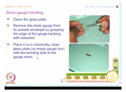
And that surface should be chemically clean that is why we have taken a glass plate or you can also use it on an empty gauge box and you also put the terminals and ensure that you keep it in such a manner that the bonding side of the gauge is down.
