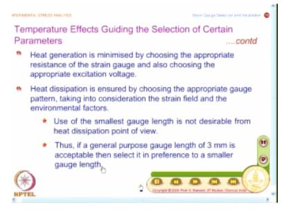
And we have looked at there are various methods to address the temperature effects and that also guides in a way how to go about in selecting a suitable strain gauge. So, the idea is what; you need to have the heat generation to be minimised. How do I minimise the generation of heat? You can choose an appropriate resistance of the strain gauge and also choose the appropriate excitation voltage.
