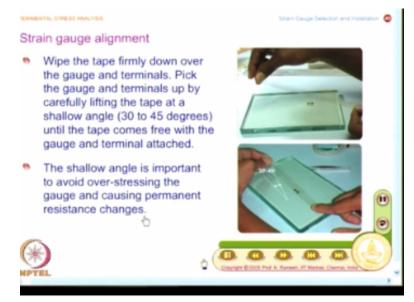
So, now you handle only the long cellophane tape with the strain gauge attached for you to align, so I can align it appropriately and you also do that practice. On the actual specimen, what you do is you put it and align it and then only go for actual bonding and this is emphasised the shallow angle is important to avoid over stressing the gauge and causing permanent resistance changes. Though this is trivial information this needs to be adhered to.
