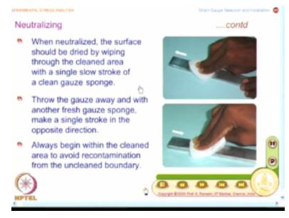
And this can be done by applying ammonia water liberally to the cleaned surface and scrubbing the surface with a clean cotton tip applicator that is what you do here and here again, you must keep the surface wet with neutraliser and as before wipe it dry with the slow stroke of clean gauze sponge, you know, though it looks very detailed set of instructions in the interest of perfect strain gauge installation, you should not get bored with this.
