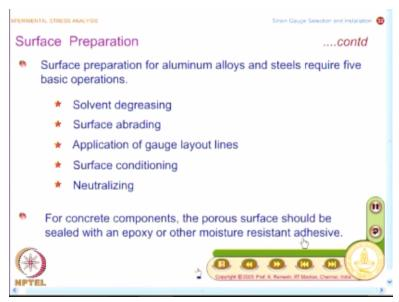
You know, before we get into the detailed steps, you need to know why we do this, we want a chemically clean surface, we want an appropriate roughness and we also maintain alkalinity of the surface for proper bonding and we also need layout lines. So, this specifies; what are the various steps that we may have to come across and if you look at for aluminium alloys and steels, the surface preparation required 5 basic operations.
