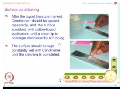
Because idea is we want to get an accuracy of 0.5 micro strains, how do I ensure that? An every step which you do has an influence on the final performance of the strain gauge system and once you put the graphite line, you know, you need to remove that carbon, so you apply conditioner and use cotton tip applicators until a clean tip is no longer discoloured by scrubbing, so this is what you do.
