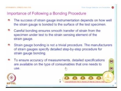
You should not mix up the STC gauges meant for aluminium, you should not paste it on steel, you should select the STC gauge meant for aluminium separately and also for steel separately and use it carefully. Now, we have all selected the strain gauge for our given application, the next important step is to bond the strain gauge to the specimen concern and this is a very, very important step.
