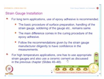
So that, you use them effectively, so what do you want to do is; we will look at how to do strain gauge installation and essentially I will be discussing how to paste a strain gauge using a quick curing adhesive such a cyano acrylate and whatever we discuss, this is also extendable to epoxy adhesive, the difference is in the epoxy adhesive. The basic procedure of surface preparation, handling of the strain gauge, soldering of the strain gauge etc. remain same.
