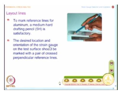
And the next important step is to put the layout lines and to mark, you can even use a drafting pencil for aluminium but for steel and other the materials, graphite pencil is not recommended, we will also see that. So, the idea of putting the layout lines is to mark the desired location and orientation of the strain gauge to be pasted. So, if you look at a strain gauge strain, gauge comes with the carrier, which has marks.
