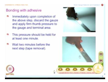
And this you need to hold it for about a minute and the bonding is complete. So, immediately upon completion of the above step, discard the gauze and apply firm thumb pressure to the gauge and terminal area, so this is how the strain gauge is bonded and you need to wait 2 minutes before the next step that will take it up later but what I will do is; I will repeat the animation for you to appreciate the sequence involved.
