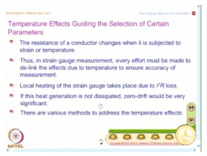
We have seen about 5 to 6 steps, we will continue in that direction and I have always been mentioning temperature effects have to be handled carefully in strain gauge technology. Though I have mentioned it several times, is no harm in mentioning it again and we will also have to look
