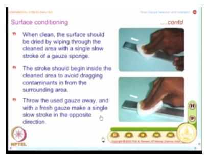
And here again, you should maintain constantly wet; the surface should be constantly wet with conditioner until the cleaning is completed because you do not want to allow the conditioner to evaporate, you keep it wet and as seen before, you need to wipe it dry, there is also a recommendation, how to wipe it. It is not that you go and then wipe it like this, you should not do back and forth.
