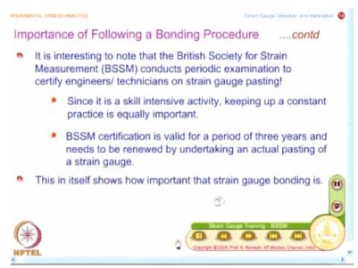
So, to ensure accuracy of measurements, detailed specifications are available on the type of consumables that one needs to use in surface preparation, bonding etc., so, it is not trivial and you have the follow the recommendation and this is very important to note that the British Society for strain measurement conducts periodic examination to certify engineers or technicians on strain gauge pasting.
