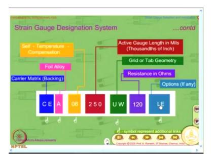
And finally we will look at what are all the options available. We have looked at carrier matrix, we have looked at foil alloy, you have already seen what is self-temperature compensation. Then you have the gauge length, grid pattern we have seen, the idea is to show a variety of strain gauges possible. Then you have resistance in ohms and what are the options.
