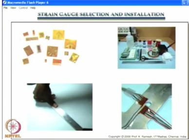
And when you go for strain gauge selection and installation you have various patterns available and for a plate with a hole you have a strip gauge that is pasted here and this shows what are the accessories that you require for strain gauge bonding and this gives an illustration how do you use a cyanoacrylate cement, what kind of procedure that you need to adopt to effect a bonding.
