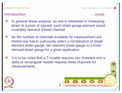
You do not have any interpretation to such type of connection. So the distinction is in general stress analysis, one is interested in measuring strain at a point of interest, that is the focus.
