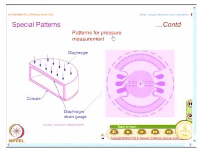
You have a special pattern for pressure measurement. I have a thin diaphragm and I have a strain gauge, which is shaped in this manner. Because I use a metal foil and then I do an etching process, I can put any complicated pattern for me to do the etching and you have one set of patterns, which are radial like this. What is a component of strain that this will sense? It will sense the radial strain because it measures only strain along the gauge length.
