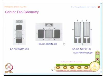
And obviously the simple strain gauge what you have is a simple loop like this and what I shown here is you have the tabs on either end and for this the particular manufacturer gives this as DN. So E denotes the carrier backing, A denotes Advance alloy and XX denotes depending on the specimen material I will have to select my self-temperature compensation number that is why this is not listed.
