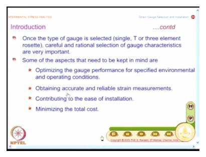
So your design can be way off, so the recommendation is combine the use of whole field technique and a point by point technique. So once you decide yes I need to have in these locations a single strain gauge, a T-rosette or a 3 element rosette, you have to make a careful and rational selection of gauge characteristics for the given application and what are the aspects that you need to keep in mind?
