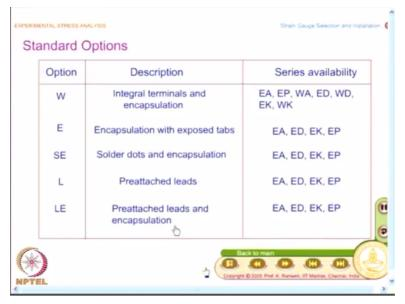
So when you look at the options, you know I have W which is integral terminals and encapsulation and when I have L it is like preattached leadwires and if I put LE it is preattached leads and encapsulation. So the idea is to emphasize for special applications, look for suitable options to minimize your effort in installing the strain gauge. So that is what we have looked at.
