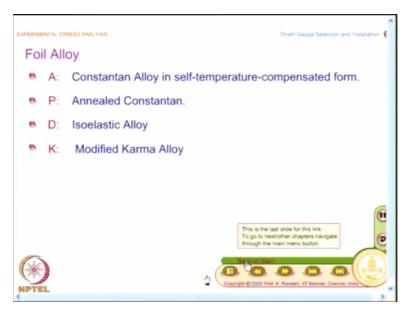
You should be able to find out what these strain gauges are in reality and A denotes Advance, it is a Constantan alloy in self-temperature compensated form, P is annealed Constantan, D is Isoelastic alloy and K is modified Karma alloy so by looking at this we will also know what is the foil alloy I am using and you have already noted you know what is the self-temperature compensation number for various specimen materials.
