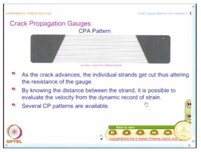
So what do you have here, in one foil I have several strands shown here. So what will happen? As a crack advances, the individual strands get cut thus altering the resistance of the gauge. So use the same principle, you are not measuring strain but you are measuring crack propagation, very interesting because I know that distance between the strings. So I can also find out the velocity.
