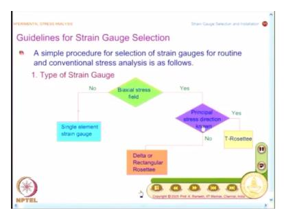
And now we will look at a generic recommendation on how to select a strain gauge for a given application. What is a first step? The first step is what is a type of strain gauge that I need at a point of interest. I have to as the question, am I working on a biaxial stress field? If the answer is no, it tells me it is enough I use a single element strain gauge.
