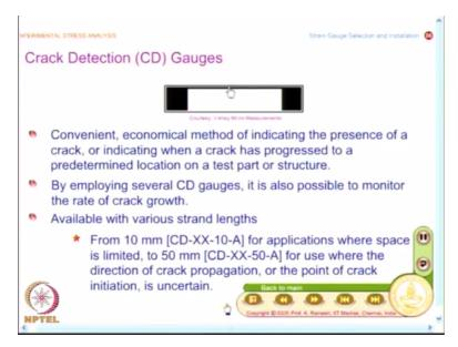
And you also have because you have an etching process, you also have special gauges. These are not essentially meant for strain measurement because fracture mechanics is becoming very, very important. You also have what are known as crack detection or CD gauges. The principle of operation is simple. Suppose I have a crack and this crack crosses the strain gauge, it will cut the element.
