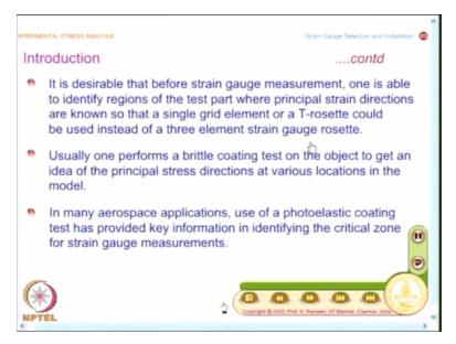
So the recommendation is it is desirable that before strain gauge measurement, one is able to identify regions of the test part where principle strain directions are known, so that a single grid element or a T-rosette could be used instead of a 3 element strain gauge rosette. You know this is the reason why we discussed the method of brittle coatings before strain gauges. Primarily, brittle coating gives you contours of isostatics.
