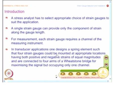
So as a stress analyst, you have to select appropriate strain gauges to suit the application and I have always been mentioning that a single strain gauge can provide only the component of strain along the gauge length and for measurement each strain gauge requires a channel. See from a large installation point of view, you may need to find out strain at several points on the object.
