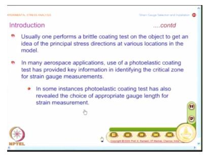
Other aspect is when you are looking at the fringe patterns, the fringe patterns also give an indication of the gradient. If the fringes are very dense then you have a very sharp variation of strain values. So you can also make some assessment on the choice of appropriate gauge length for strain measurement. See this is the general thumb rule.
