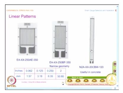
And the idea here is to show a variety, you know I can have a very wide grid pattern. Why do you have the wide grid pattern? For heat dissipation. A heat dissipation is an issue then go for a wide grid. Otherwise go for a narrow grid and this is other extreme, you have a very long strain gauge. You have to know that such strain gauges are really available and this is about 50.80 millimeter.
