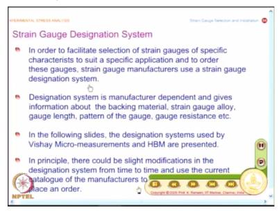
And you know if I have to select a strain gauge of suitable characteristics and also to order these gauges, strain gauge manufacturers use a strain gauge designation system. So it does 2 jobs, one is to facilitate selection of strain gauges or specific characteristics and also to order these gauges and obviously the designation system is manufacturer dependent and gives information about the backing material, strain gauge alloy, gauge length, pattern of the gauge, gauge resistance etc.
