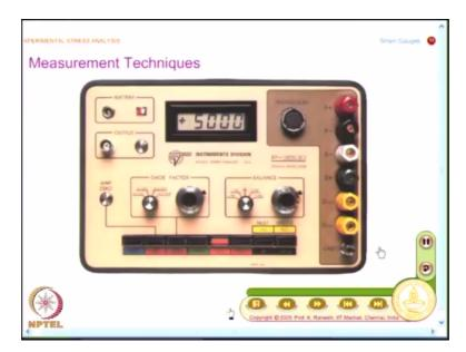
Now we go and look at what are the measurement techniques. I am showing a typical strain gauge meter and I would like you to draw your attention to few finer aspects. First issue is if you look at very carefully, this is for 120 ohms and this is for 350 ohms. It may not be clear on the screen but you know there are provisions available for selecting internal resistors of 120 ohms or 350 ohms.
