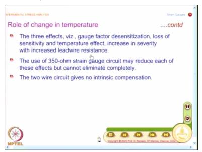
So what you find is the gauge factor desensitization or loss of sensitivity and temperature effect increase in severity with increased leadwire resistance. So you have to account for it in practical applications. So one way of looking at this is going for a 350 ohm strain gauge. This
