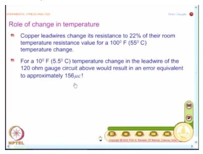
And it is noted that copper leadwire change its resistance to 22% of the room temperature resistance for a 55 degree centigrade temperature change. So if there is a change of 55 degree centigrade, the resistance will change by 22%. We will not look at a change of 55 degree centigrade. We will just look at a change of 5.5 degree centigrade change in temperature. If I
