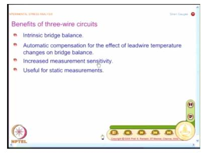
And what are the benefits of 3-wire circuits? A 3-wire circuit has intrinsic bridge balance. It has an automatic compensation for the effect of leadwire temperature changes on bridge balance and it also has increased measurement sensitivity and definitely recommended for static measurements because temperature effects are significant when you are measuring over a period of time.
