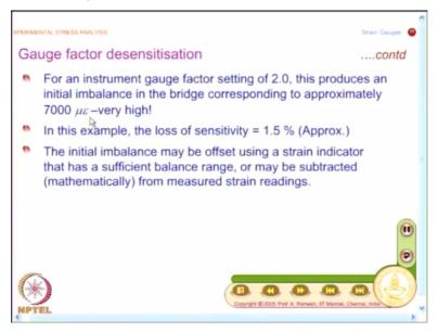
When I have 1.7 ohms, I find the equivalence in terms of strain is 7000 microstrain and we have already seen in the case of most engineering materials 0.2% strain the material yields, 0.2% is 2000 microstrain so we will never go to 7000 microstrain unless I am looking at some plastic deformation and so on. So my measurement range will be much smaller, so this is what you have to keep in mind.
