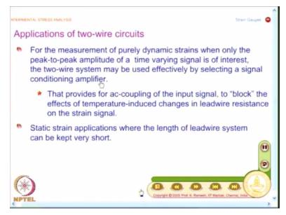
We will see in which class of problems the 2-wire circuits are applicable. Suppose I am working only on dynamic strains when only the peak-to-peak amplitude of a time varying signal is of interest and in such applications, the 2-wire system may be used effectively by selecting a signal conditioning amplifier. The conditioning amplifier need to provide for accoupling of the input signal, to block the effect of temperature induced changes in leadwire resistance on the strain signal.
