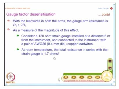
And as I mentioned earlier the resistance in that arm increases to RG+2RL and let us look at a simple practical example. Suppose I take an installation which is at a distance of 6 meter from the instrument and you have to connect this strain gauge to the instrument and you take a good set of copper leadwires, the specifications also given, this is AWG26 of 0.4 millimeter dia.
