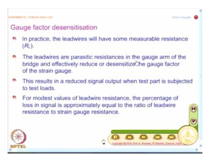
And what way it modifies your measurement of strain. You will have to note that leadwires are parasitic resistances in the gauge arm. You do not want them, you want to have a magic material which has no resistance and strain gauge is connected. See I also said if you have a magic material, a single spec of it can have 120 ohms or 350 ohms, I paste it at the point of interest and connect it and make measurement, then I have no problem about strain variation or gauge length influence etc.
