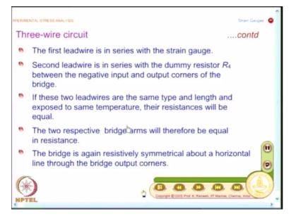
And whatever I have said earlier is now summarized as points. The first leadwire is in series with the strain gauge. The second leadwire is in series with the dummy resistor R4 between the negative input and output corners of the bridge. So I have leadwire on 2 different arms and obviously you are going to have these 2 leadwires of the same type and length and exposed to same temperature, the resistance will be equal.
