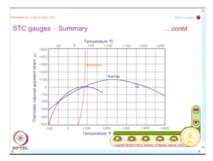
And the suggestion is I have temperature and I have thermally induced apparent strain. So I measure from this graph for a given temperature what is a thermally induced apparent strain and subtract it from my measurement. Whatever the measurement I make, I subtract it, but this is cumbersome.
