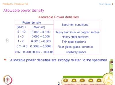
So this is what you have to look at allowable power densities are strongly related to the specimen that is what this table essentially brings out. So in a strain gauge installation, I said strain gauge
