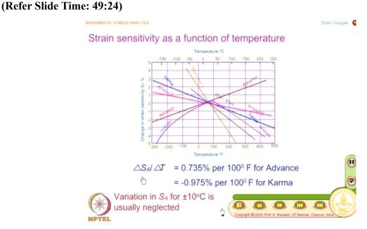
And what you find is fortunately it is the linear graph, for the popular strain gauge material like advance, karma, as well as high temperature applications like nichrome, armour D, as well as the platinum tungsten type of strain gauge alloy, only for isoelastic it is non-linear. So if it is linear, it is good enough. So you just make a note that advance and karma it is varying linear that is what you need to worry about, itself variation is linear, fortunately, it is linear.
