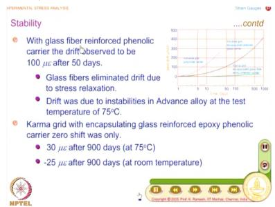
Now I go and improve the carrier instead of polyamide if I use the glass fiber reinforced phenolic carrier, the drift has reduced from 270 microstrain to 100 micro strain, even after 50 days. In fact, that is what is listed in this graph, this is about 270 microstrain, this you see at the end of 30 days and at the end of 50 days, you find only a 100 micro strain, by just changing the carrier for the strain gauge. So whatever the stress relaxation, the glass fibers eliminated that effect.
