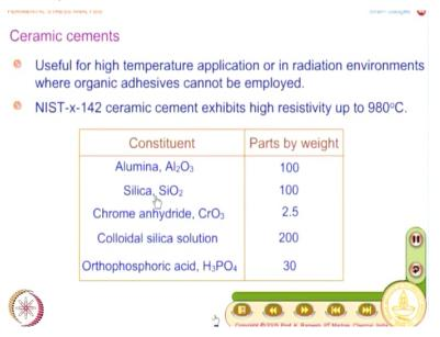
And when you look at ceramic cements, they are useful for high temperature application or in radiation environments. See now nuclear power is becoming very very important, so you need to live with radiation environments in such installations. And in such applications, organic adhesives cannot be employed, so you need to necessarily go for ceramic cements. And one of the popular ceramic cement is NIST-x-142, which exhibits high resistivity up to 980 degree centigrade.
