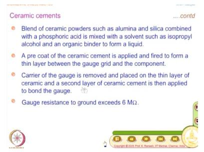
So what you have here is, you have the blend of ceramic powders such as alumina and silica, combined with the phosphoric acid is mixed with a solvent such as isopropyl alcohol and an organic binder to form a liquid. So essentially you have the ceramic available as a liquid, so that it is easy for you to apply it by a spraying process. And what you do is on the specimen, you provide a pre-coat of the ceramic cement.
