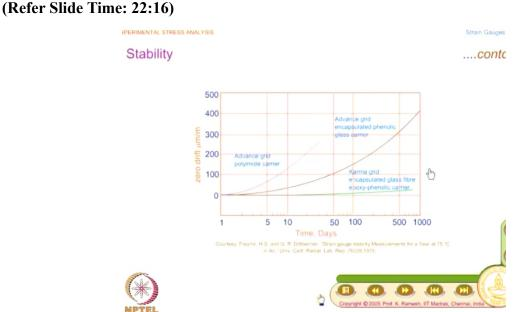
I have a graph, which shows time versus zero shift time is plotted in a log scale I have 10 days, 100 days and 1000 days. And I have three graphs, I have one graph for strain gauge alloys advanced grid and polyamide carrier, and the second graph is the grid material is same, it is again advanced grid, encapsulated phenolic glass carrier, the carrier is made different. You have the encapsulation and you have the phenolic glass carrier, it is much better than the polyamide carrier.
