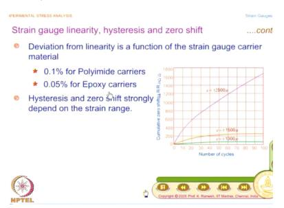
And what I have here, suppose I want to minimize deviation from linearity, then choose an appropriate carrier. What you find is polyamide carriers the deviation is about 0.1%. On the other hand, if I go for epoxy carriers, it is just half of it, it is about 0.05%. But you know very well, polyamide is easy to handle. It is a plastic, even a beginner can handle this polyamide carrier. We have already looked at epoxies brittle that is recommended for transducer applications.
