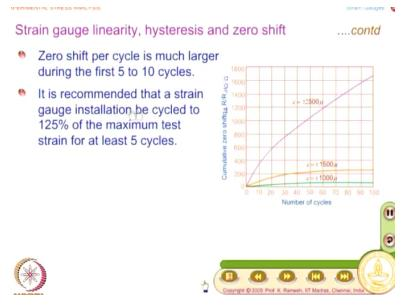
The recommendation is we find that the zero shift changes in the initial few cycles, so you have zero shift per cycle is much larger during the first 5 to 10 cycles that is what the graph shows. So what you do is, it is recommended that a strain gauge installation be cycled to 125% of the maximum test strain for at least 5 cycles. So you do not go and make the measurement as soon as you paste it, and the strain gauge is ready for measurement.
