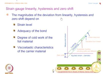
And we have already look at you need to worry about strain gauge linearity, hysteresis and zero shift in any strain measurement application. And what happens to the magnitudes of these like deviation from linearity, hysteresis and zero shift, they all depend on various factors. What is the
