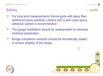
See what you have here is for long term measurements, karma grids with glass fiber reinforced epoxy phenolic carriers, with a well cured epoxy adhesive system is recommended. I said that adhesive has not be mentioned, but what you find here is for any sophisticated applications, people go for epoxy adhesive. And you should also ensure that the gauge installation is water proofed well. You do this to minimize moisture penetration.
