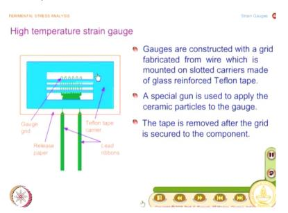
And you have an example of a how such a gauge can be constructed. I have a sketch here, I essentially have a wire type strain gauge, and you have a Teflon tape carrier, which could be peeled off, and you make a decent sketch of this. So what you have here is gauges are constructed with a grid fabricated from wire, which is mounted on slotted carriers made of glass reinforced Teflon tape.
