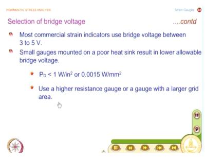
So how I go about and select the bridge voltage? If we look at most common strain indicators, use bridge voltage between 3 to 5 volts. Small gauges mounted on a poor heat sink result in lower allowable bridge voltage. So there is the reason, when we had a discussion on selection of gauge length, we saw if the strain is varying linearly, length of the gauge length do not matter in interpreting the strain at the center of the strain gauge.
