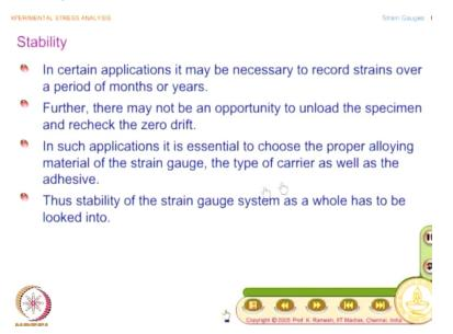
Now we get on to another important issue in all strain gauge installation that is stability, this become very important in applications, when you have to record the strains over a period of months or years, it is not just that you do the strain measurement for immediate requirement, and forget about it. Suppose, I want to monitor structures like dams and bridges, we may have to do it for long periods of time.
