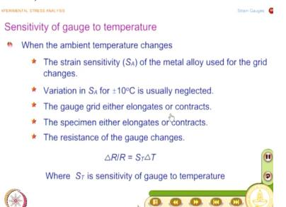
Now we have talked about influences of temperature, in some form you should also look at what is the sensitivity of the gauged temperature, what happens when the temperature changes. The strain sensitivity SA of the metal alloy used for the grid changes. We will have to see, how does it change? That is the question. And for simplification for a change of + or - 10 degree centigrade, the variation of SA is usually neglected.
