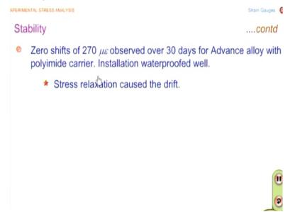
And what you find here is, a zero shift of the order of 270 microstrain is observed after 30 days for advance alloy with polyamide carrier. And if you look at the installation, installation was water proofed well, there was no difficulty of moisture entering into it, and deteriorating the strain gauge bonding. And what people found was the carrier is not taking the load properly, so there was stress relaxation, which has caused the drift.
