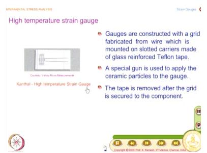
And they have what is known as Kanthal which is meant for high temperature strain gauge, and you could see the slotted Teflon tape carrier, and you have the strain gauge available like this, so this can be used to put the ceramic cement, and remove the carrier, and put another layer. So essentially you will have only a ceramic base and you have a metallic foil, there is nothing like a polymer that comes in between.
