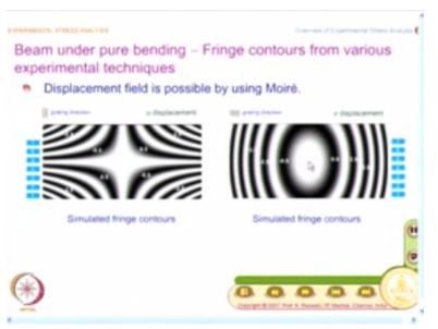
What I can do is I can do a contour, I can look at geometric Moire and find out how the displacement field is and this is what the U displacement and this is what the V displacement and we would see this little closely.
