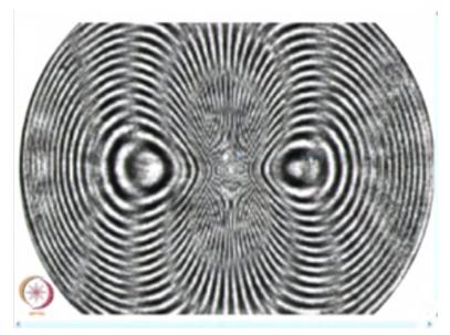
What you see here is I have on the background slope fringes. On the slope fringes, you see faintly the curvature fringes, right. When I have shown sigma 1-sigma 2 contour superimposed with isoclinics, you felt uncomfortable. Now, you will say that was much better because it had very good contrast. Here I get curvature information but the advantage here is though it looks little dull, the advantage is the optical arrangement used gives both slope and curvature information in one shot.
