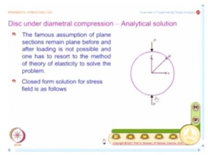
Now, the next problem is we move onto disc under diametrical compression and that is what shown here. I have the disc and the centre of the disc is taken as the origin. I have X and Y coordinates and R is the radius of the disc. I have a diametrical load P which is acting on it and we will call this diameter as either D or d and for this problem you have closed form solution from theory of elasticity.
