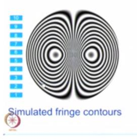
What you have here is I increase the load. So, people also say this as butterfly fringes, they look like the wings of a butterfly and they call this as butterfly fringes, particularly in the case of non-restrictive testing, when I want to do a honeycomb panel testing, any delamination you would be able to find out easily. If you see butterfly, you should not feel happy, you should feel disturbed that there is a delamination.
