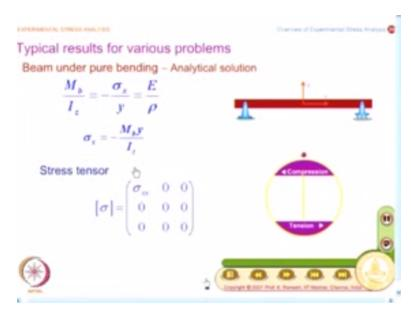
Now, we take up the problem of beam under 4-point bending and what you have here is, I have a beam and this is shown as X axis, this is Y axis and you have taken central portion of the beam which is subjected to bending moment M, B and in this you have the stress variation over the depth as like this which shows the variation is linear and central core does not contribute to load shearing.
