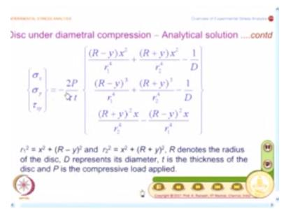
Fortunately, theory of elasticity provides the solution. Here again it is given in a convenient form, sigma X, sigma Y of XY and you have this as -2P/pi T and I would request all of you to take down these equations. Though these equations are very long, they are very valuable information. When we develop photoelasticity, we could directly use these equations for our interpretation and you have sigma X R-y x square/r1 power 4 and r1 is defined as r1 square=x square+R-y whole square.
