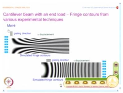
What you have here is I again have a grating direction and knowing this grating direction, it is possible for you to say it is U displacement. Knowing this grating direction, it is possible for you to say this is V displacement and you also have a feel of doing the experiment by seeing what happens as a function of load. I gradually increase the load and more and more fringes get formed and you could make a simple sketch of it, try to get only the skeleton, you do not have to draw the band.
