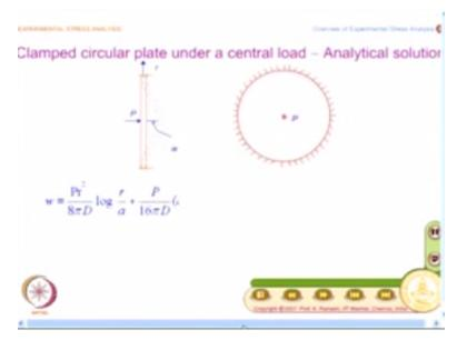
The next problem what we would take on is, we would take on the problem of a clamped circular plate under a central load and what I would appreciate is I have this clamped circular plate. This is clamped all around the periphery and is subjected to a central load. In fact, in the kind of problems where they do out-of-plane displacement, they take this as the benchmark example and using this only they testify their methods.
