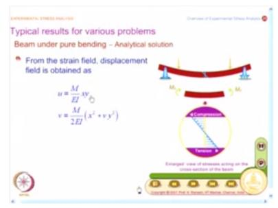
We will see the fringe pattern. It is will a second for it to come and what you will see is when I magnify it, you will see in a very subtle fashion what you have on the top fibre. In this particular fibre, the top fibre is subjected to compression and bottom fibre is subjected to tension. So, you will have the fringe order slightly greater than what is there at the bottom. So, it is not perfect symmetry. So, the experiment captures this,
