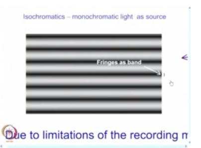
Now, what I do is I take the model put it on optics and find out what the contours look like. I do not get straight lines as thin as possible, I get only a band. I get essentially straight bands. So, this result matches with what you have seen in analytical solution with a difference. The difference is I see the fringes as a band rather than a single line and I see this as black-and-white contours mainly because I have used monochromatic light source for elimination.
