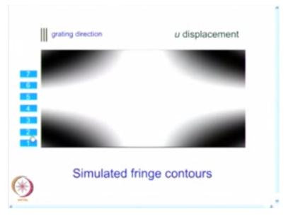
There is many indirect learning you learn, one is suppose, I change load and you see this is how the fringes are developed. As the load is increased more and more, fringes are developed and this is a very key information in most of the experimental techniques to label the fringe orders as an auxiliary method to do that. Another one what you find is the fringe thickness is different. This also carry some information. This we will see later part of the course.
