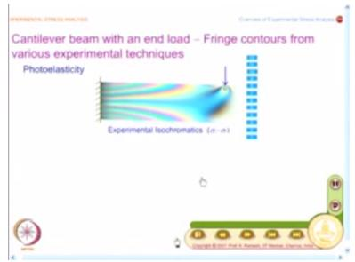
So, first thing what we have always been doing is photoelasticity and you all know that it gives you contours of sigma 1-sigma 2 and these contours you would not be able to calculate right at the class. It is better that you have computer software to evaluate it and also have a post processing where you can go and plot it. As before, I would like you to have a reasonable sketch of these fringe patterns.
