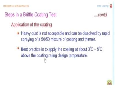
So, when you face a problem you always have a solution heavy dust is not acceptable and you can dissolve it by rapid spraying or 50/50 mixture of coating and thinner. So, this is the beauty when you look at the procedure you know the manufacturer has looked at all aspects of applying the coating. Because in all coating techniques only if the coating is properly formed data interpretation is meaningful.
