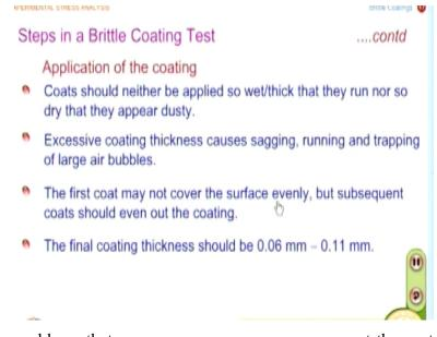
And what are the problems that you can come across see you want the coat should neither be applied so wet/thick that they run nor so dry that they appear dusty. So, it has to be in between totally wet and totally dry. And what will happen if you have excessive coating thickness excessive coating thickness may cause sagging, running and trapping of large air bubbles. See this is very important when you are applying coating.
