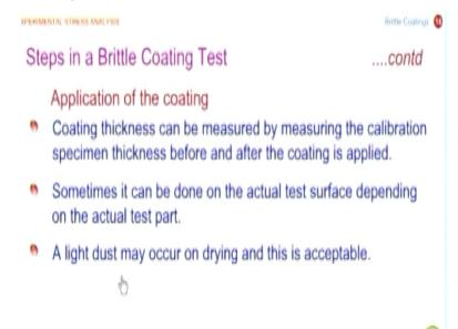
So, one way of looking at that the thickness is to measure the calibration specimen thickness before and after the coating is applied. So, this is straightforward because you are keeping the calibration specimen as part of your specimen preparation. So, whatever the operation that you do for the specimen is evenly done for the calibration specimen. If you have done 5 passes on the actual specimen, you also do 5 passes on the calibrations specimen.
