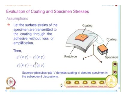
And the assumptions are also similar so I have a prototype I have a coatings and on the coating a select appropriately a axis for convenience I take axis 1 and 2 they correspond to the principal strain direction at the point of interest and what we assume is the coatings strain=the specimen strain at that point of interest. The adhesive is properly used to transfer the strain without loss or amplification.
