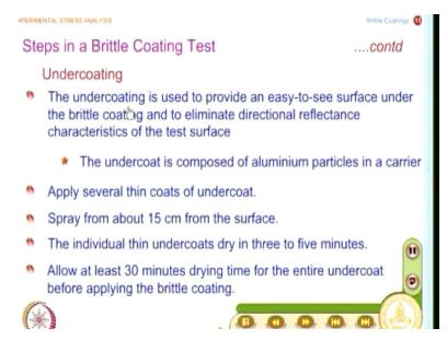
The third step is to provide them undercoat and what is the use of the undercoat, undercoating is used to provide an easy to see surface under the brittle coating and to eliminate directional reflectance characteristics of the test surface. It is very important because you have to go and identify the cracks and you must have the convenience in detecting the cracks and what is the type of undercoat they have the undercoat is composed of aluminum particles in a carrier.
