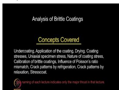
Let us continue our discussion on brittle coatings we saw one of the earliest brittle coatings was naturally formed scales on hard cold steel and the author saw even the oxides that were formed on surfaces there were also used as a brittle coating. And primarily those coatings fail to indicate the presence of plastic deformation in the component. Only later with advancement in material research people developed sensitive coatings which fail at strains much below the yield strain.
