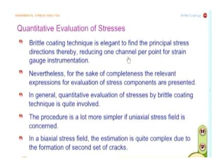
Now let us look at how do I do quantitative evaluation of stresses. And this is what I emphasize again and again brittle coating technique is elegant to find the principal stress directions thereby reducing 1 channel per point for strain gauge instrumentation. And I have already indicated to some extent that quantitative evaluation of stresses by brittle coating is quite involved. On the other hand, suppose I have only a uniaxial stress field on the specimen.
