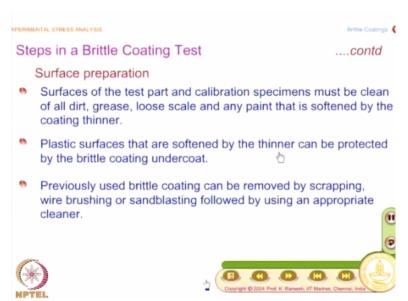
And the next step is what? In all the coating techniques surface preparation assumes important. You can actually abbreviate this and write it rather than writing full sentences like what I have wrote here. And when I have to bond a coating the surface must be clean of all dirt, grease, loose scale and any paint that is softened by the coating thinner. So that has to be done. Then what you have is you have plastic surfaces.
