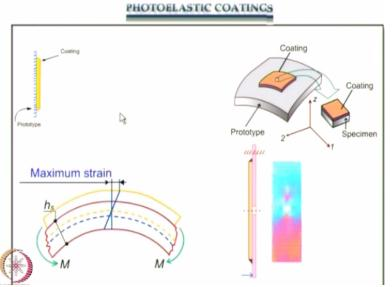
In summary, what you can look at is you have a simple optical arrangement then I said for all coating techniques the coating has to be bonded very carefully on the prototype and we also assume that strains are faithfully transferred from the prototype to the coating. And I said once you come to Photoelastic coating you have to think of what are known as correction factors, that is what is illustrated here.
