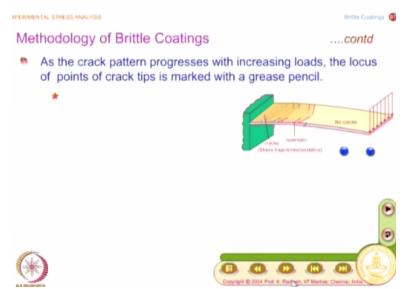
And then take a closer look at it. I have this and I also zoom it further, so what you have here is the isostatics or parallel like this and you see isoentatics of different colors which is for different loads. And what is important is then do the first set of cracks formed. It is very important. I have to be careful in deciding my load increments. So in this experiment you see isostatics as well as isoentatic.
