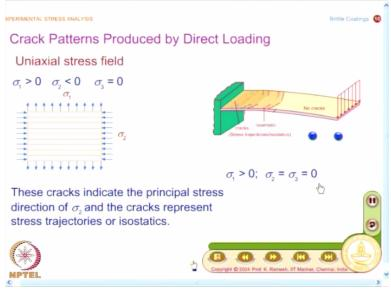
Now we look at what kind of crack patterns formed by direct loading. And this is what is shown here. Suppose I have sigma 1 is > 0 and sigma 2 < 0 and sigma 3 = 0, I have essentially a biaxial loading situation and sigma 1 is > 0, so you have cracks formed perpendicular to the direction. So by looking at that crack formed I can comment that this is a combination of uniaxial stress either I can have uniaxial stress or you have a tension compression.
