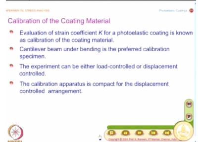
Now we move onto the important aspect that we have to do as part of the photoelastic coating test is. How to calibrate the coating material? And what is the meaning of Calibration? Evaluation of strain coefficient K for a photoelastic coating is known as calibration of the coating material. And if you look at what is most preferred calibration specimen is the Cantilever beam under bending.
