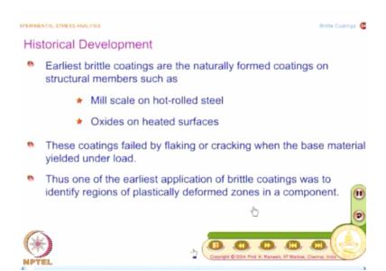
And, we have already had a bird's eye view of what brittle coating is in one of the initial lectures. You know very well that you have a coating that is put on the specimen which is brittle in nature. And this coating is allowed to fail under the application of the load and we also looked at what are ISO tactic and ISO entotic. We will see that in more detail.
