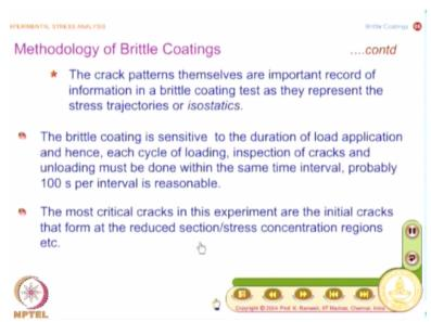
And this is what I have been emphasizing it again and again. The crack patterns themselves are important record of information in a brittle coating. They are represented and they represent the stress trajectories or isostatics. So people have developed methodologies to inspect for appearance of cracks. They have very elaborate methods – several methods are available so that you do not miss any zone where cracks are being formed.
