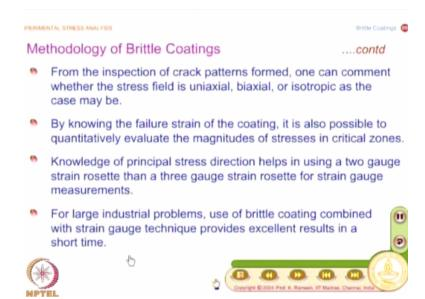
And what is important is like in optical techniques here also I see whole field information. By looking at the crack patterns formed, one can comment whether the stress field is uniaxial, biaxial, or isotropic. In fact, in some of the earlier studies even to identify zones of uniaxial, biaxial and then isotropic was an issue. It was a large problem. Suppose I know in a particular region I have only uniaxial state of stress then I can reduce the strain gauge channel that is the advantage.
