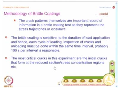
So that is what again emphasized. You need exercise considerable care in obtaining the load at which the initial cracks initiate as they represent zones of high stressed regions. See the methodology is like this. The coating is designed to fail at a particular strain level. If the crack has formed at a given load what it indicates is the strain level is at least this, it could be more than that also.
