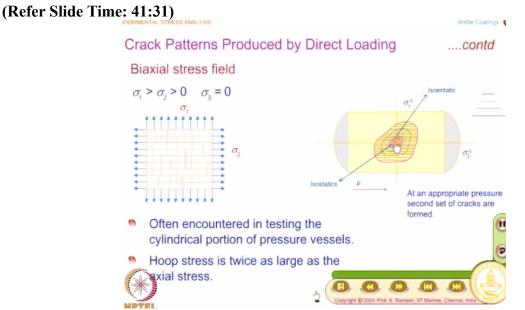
Suppose I have a tension, tension combinations, what happens? And where they have this tension-tension combination in your engineering? See engineers always deal with the pressure vessels. And once you deal with the pressure vessel you have Hoop stress as well as longitudinal stress, this is a very nice example where tension-tension combination exists, not only this, you know Hoop stress is much larger than the longitudinal stress. So only when the pressure is sufficiently increase.
