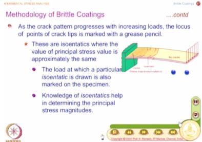
And what you have is the crack pattern progresses with increasing loads, the locus of points of crack tips is marked with a grease pencil. We will see that with the example.
