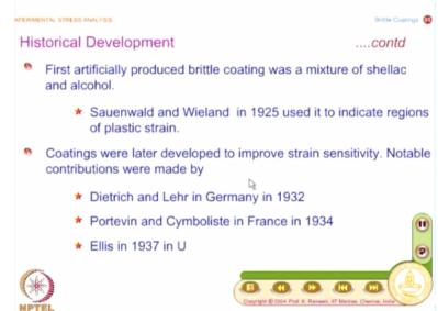
And it is desirable to look at what are the contributions by various scientists. And it is also interesting to see what was the first artificially produced brittle coating. We have seen naturally formed coatings earlier. The first artificially produced brittle coating was a mixture of shellac and alcohol. And this was used by Sauenwald and Wieland in 1925 to indicate regions of plastic strain.
