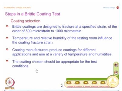
And you know, once you come to a Brittle Coating test the first step that you need to do is you have to select a coating. And if you look at any brittle coating test any supplier who supplies coatings he gives a different set of coatings for a variety of temperature and humidity. So depending on your test conditions you have to choose the coating that is appropriate for the test conditions. And I said (()) (48:00) is very, very sensitive.
