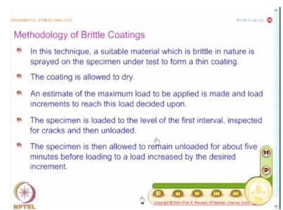
And what is the methodology of Brittle Coatings? This you already know, we are only going to refresh our old memories and in a very formal sense. So what I have is, in this technique, a suitable material which is brittle in nature that is the key point. And what way it is bonded, it is sprayed on the specimen under test to form a thin coating. So this simplifies your specimen preparation. Because I can cover large areas by a spray gun.
