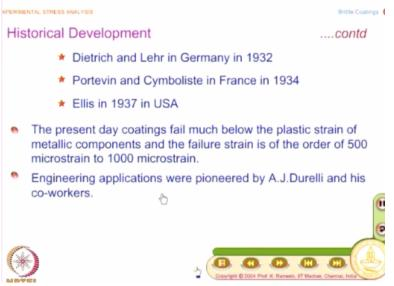
And the present day coatings fail much below the plastic strain, that is what you have to look at. It started with identifying zones of plasticity in a model and failure strain is of the order of 500 to 1000 microstrain even less. Now people say even 300 microstrain possible. So you have material research contributed to development of better coating materials which have more sensitivity for failure. Here the coating as to fail. The coating has to fail by microstrain.
