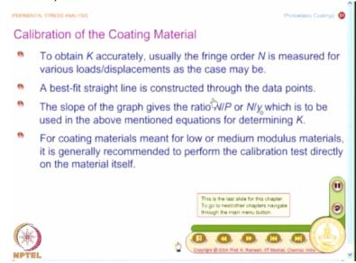
And you know, I have been saying that in photoelastic analysis the calibration constant has to be determined as accurately as possible. The same rule applies to evaluating K as well. It has to be obtained a accurately as possible. So for this you need to find the fringe order correctly and you just do not make one measurement you make various for various loads and displacement find out the fringe order, and do a graphical least square analysis.
