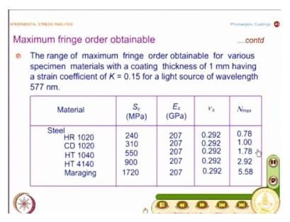
And I also have a table which gives you for a variety of materials what is the fringe order obtainable and what you have is we have taken a coating material of K=0.15 and for a coating thickness of 1 millimeter and for a light source of wavelength 577 nanometer. Essentially the white light we had also looked at the color code where we saw repetition occurs at 577 nanometer you have a tint of passage and twice of this value you have another tint of passage.
