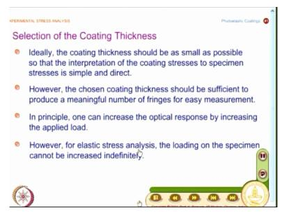
And I also mentioned there is an issue of Selection of Coating Thickness. Ideally I want the coating thickness should be as small as possible. He said we want to have a very high value of K then I can have coating thickness as small as possible and we also want to have the chosen coating thickness should be sufficient to produce a meaningful number of fringes for easy measurements.
