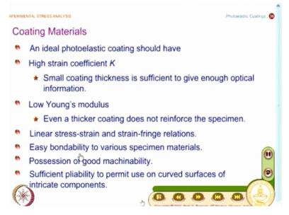
And what should be the property of ideal photoelastic coating should have. Obviously we want to have high strain coefficient K. The reason is I need to get enough optical response and we have also seen if the coating is thin enough I do not have to worry about the correction factor which is automatically taken care off only when the coating thickness is considerable then correction factors are very important.
