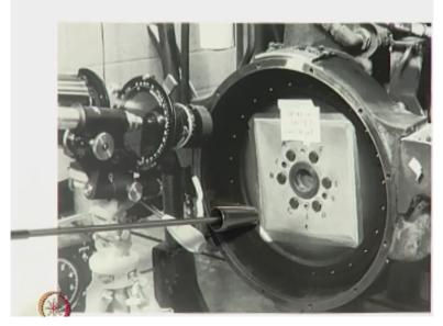
This shows another example of application of photoelastic coatings. Here you have a flywheel that is being analyzed.
