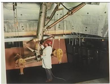
This shows another example of what is the use of photoelastic coating in solving industrial problems. This is the model of A330, A340 Landing Gear and what you have here is you can see the size of the model compared to the human being standing. And what is interesting is you have this as a epoxy model that is very clearly seen from the color you can see from the color that this is the model made of epoxy.
