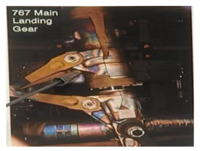
This shows another example of component of Landing Gear. This is a 767 Main Landing Gear how photoelastic coating reveals stress patterns for a problem of practical interest.
