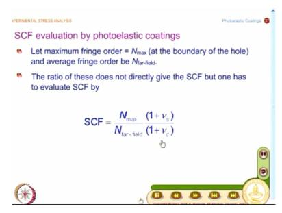
However, when we go and do the SCF evaluation that is what I said when I want to find out the stress concentration factor. Photoelasticity is a very simple approach to find out stress concentration factor. And what we need in transmission photoelasticity is you need to find out n max and n far-field and the ratio directly gives you the stress concentration factor, but in view of the Poisson's ratio mismatch you have to modify this expression slightly.
