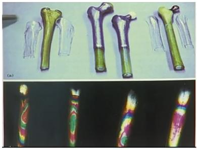
This shows another example of application of photoelastic coating and here it is for prosthesis example where you have hip replacement and you would not analyze what is the influence of this implants. You have a shell which is made by contourable plastic which is bonded on to the bone and these are all the respective fringe patterns obtain for various configuration. So you have a range you have seen for metals. Now you see for applications of photoelastic coating to bone.
