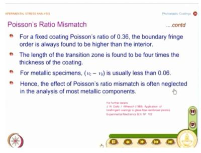
And this is what you see here and what they have found is for a fixed coating Poisson ratio of 0.36 which is reasonable to assume. The boundary fringe order is always found to be higher than the interior. It is mainly because of the Poisson ratio mismatch and their length of the transition zone is found to be 4 times the thickness of the coating. So this is the contribution by the experiments conducted by Dally, I. Alfirevich.
