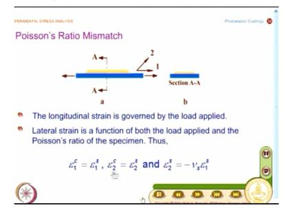
And let us understand the mismatch of Poisson ratio how does this affect. So what is shown here is I have a simple specimen subjected to uniaxial tension. I take axis 1 along this specimen. I take axis 2 traverse to the specimen and I have a photoelastic coating pasted on this. And if you take a section here I show the section will look something like this. It is deliberately shown that you have this coating interior it is not extended to the full length to illustrate the point.
