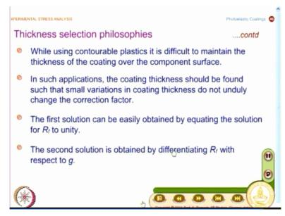
And that is what is summarized here while using contourable plastics it is difficult to maintain the thickness of the coating over the component surface. So in such applications the coating thickness should be found such that small variations in coating thickness do not unduly change the correction factor. In fact, we are going to see a variety of problems which are very complex in shape where contourable plastics have been employed to analyze a variety of practical situations.
