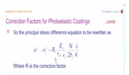
It is not as simple as you saw in the case of transmission photoelasticity mainly because of mismatch of Poisson's ratio, which becomes significant in those class of problems and we will
