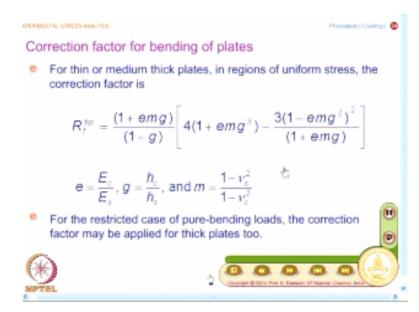
And it is subjected to bending loads, so you have to use correction factor right from calibration of the coating material, so it is very important and what are all the ways that I can use this, from whatever the expression that I have got, I could also go and extrapolate it for bending of plates, we will see a little while later. For thin or medium thick plates in regions of uniform stress, the correction factor is given as bp denotes bending of plates.
