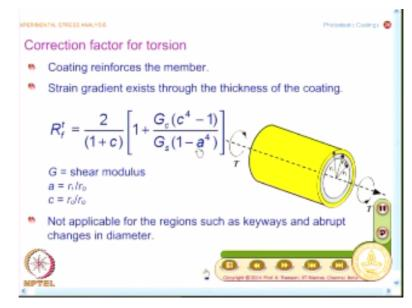
Whatever, the digital photo elastic principles, which we have learnt are also equally applicable to reflection photoelasticity, so, when I go for digital reflection photoelasticity, I can afford to use a thin coating and do my experiment. So, my nuisance from correction factor effort becomes minimal. Now, we take up, what are the correction factors in the case of torsion and I am going to give you the expression directly.
