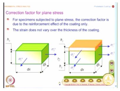
I can find out sigma 1s - sigma 2s and what we will have is; we will have this correction factor evaluated for in plane stress, bending, torsion and internal pressure so on and so forth that is how we will have. We will have different expressions for Rf and Rf is used because it is essentially a reinforcement factor and we will first take up; what are the correction factors for plane stress.
