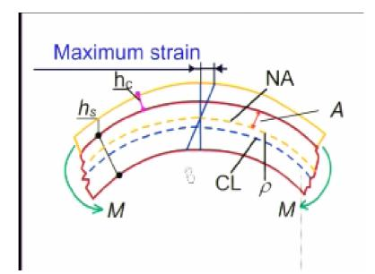
And you can also have a clear picture of the beam and to label various quantities, so you look at; I have a thickness of the specimen, I have the thickness of the coating and the neutral axis, no longer coincides with the centroidal axis of the specimen cross section but it gets shifted and we have labelled the distance from one of the ends of the specimen top surface to the neutral axis as, a and you have a radius of curvature rho.
