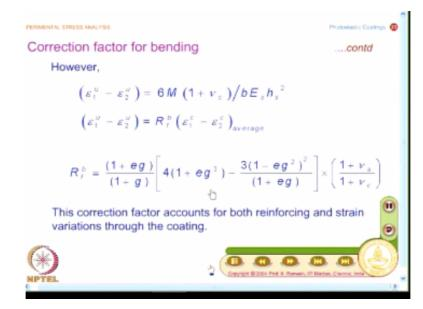
So, now you have methodology how to go about and write the final expression for correction factor in bending. I have now have expression for average strain difference and I will also related to the uncoated strain difference, then my job is done and what you have as uncoated strain difference, this behaves like a simple beam. Whereas, when I have a coated specimen it behaves like a composite beam, so this is what I have here.
