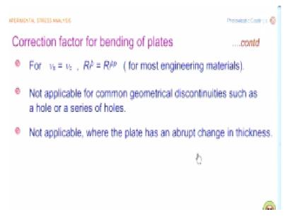
We will see now that when I have Nu s = Nu c, I do not have to separately go and find out correction factor for bending of plates, I can use simply the correction factor for bending what we had developed earlier, you know these are all the developments in the old days, where they had only slide rule to work with. Now, you have computer software available, you have to just put in your thickness of the specimen and thickness of the coating and coating and material properties.
