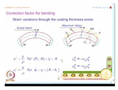
Now, we will move and find out; how do I go about for a correction factor, when the specimen is subjected to bending. So, what you have here is; if I have a specimen, which is uncoated for a given bending moment, it would have its neutral axis like this and strains vary linearly over the depth of the beam. Now, what I have here is on top of this specimen, I put a coating material then this system behaves like a composite beam.
