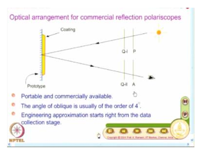
So, what is the kind of arrangement that they have in a commercial reflection polariscope. Observe the animation again, so what i have here is; I have to send the ray of light to the model and I have to analyse only the reflected light and what I can do this is; I have to do this at an angle for me, this is a reflected light. The way, I can improve my technique is keep this light source and your observation far away from the model.
