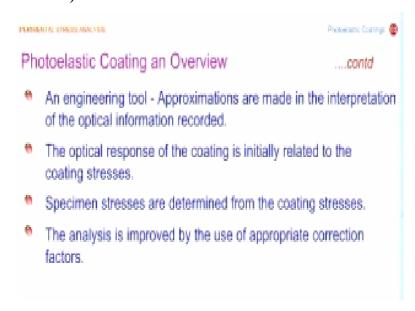
So, you are really talking about sufficient thickness, so that you have to keep in mind and you have to appreciate that this is an engineering tool and I have said engineering means approximations and approximations are made in the interpretation of the optical information recorded. We say that we want normal incidence in photoelasticity and you would find because of industrial application even that is compromised to some extent.
