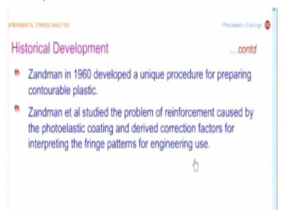
And because you see the reflected light, this is also termed as reflection photoelasticity and the other difficulty was lack of proper adhesives to bond these coating were also a problem. So, the development of the technique hinges on development of proper adhesives and also development of epoxy resins. Initially, many of these applications were confined to flat surfaces, later it was shown by Zandman, who developed in 1960.
