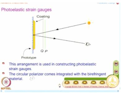
And one of the outcome of this kind of approach is also what are known as photo elastic strain gauges. What they have done is along with the coating, you will have the quarter wave plate and polarizer integrated with it, you know these were developed in Germany, like you have electrical resistance strain gauges; you will have a small strip of plastic with its own quarter wave plate and polarizer embedded.
