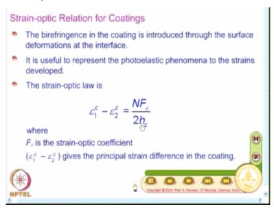
So, instead of looking at stress optic law, I should essentially look at strain optically that is more appropriate because the way the model is loaded, the way the coating is loaded is different. So, we will have to look at what is strain optic law? So, what I have here is the birefringence in the coating is introduced through the surface deformations of the interface because we said that the coating becomes temporarily birefringence, when loaded.
