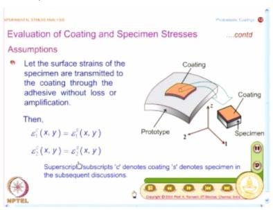
And what do we see and we also have a very nice way of looking at it, I have this as a prototype that is given in grey shape. On the prototype, I put a coating at a place of interest, which is large enough and I take a small element, which is shown here and I have a full freedom to select my
