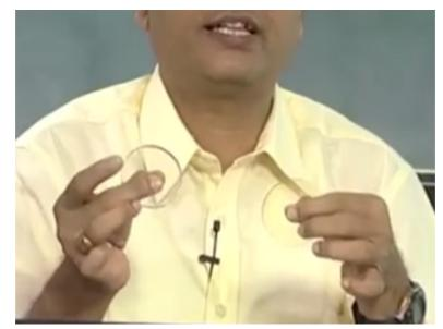
We will also see them physically and also see their properties and what I have here is I have an epoxy disc, this is the disc made of epoxy and this will have particular elastic properties and I have another model, which is made of polycarbonate. This is of polycarbonate even by looking at the difference it has a slight yellowish tinge and these properties are very similar in characteristics.
