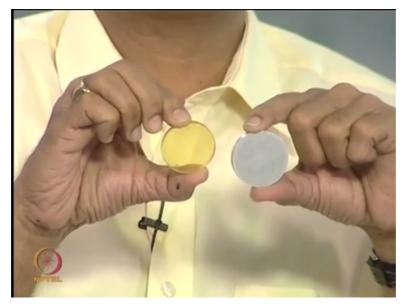
See now we come back to our famous problem, you know I have plastic model, this plastic model is polyurethane and I have an aluminium specimen and apply the same diametral compression load and what will happen to the plastic model? Plastic model will deform visibly because it has a lower Young's modulus whereas aluminium is about 70 GPa and plastic is around 3 GPa in general.
