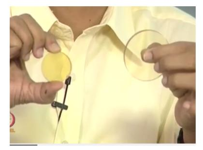
On the other extreme, I have the polyurethane model and this also has a tinge of yellow. The difference is I can even compress it with my fingers. It has such a low elastic modulus and I can compress it. You can see the deformation when it is loaded, you can see the deformation when it is compressed, you can see my fingers are pressing that it is so soft. So it is very good for models for class illustration and also a good model to do the fingernail test.
