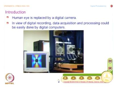
What we introduced was, in the case of digital photoelasticity, you replace the human eye by an electronic eye. You have a digital camera. These are essentially charge coupled devices. You call them as CCD camera and once you use a CCD camera, it is possible for you to get the image as an assembly of numbers.
