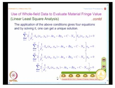
How to construct the equation that you need to know because the idea here is we want to get a unique solution. For us to get a unique solution for multiple data points, we construct only the number of equations = the number of unknowns. That is what we want to do it and this differentiation is very simple. See, normally you are differentiate with respect to x and with respect to y.
