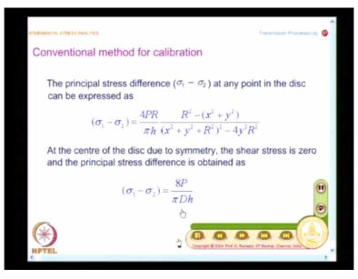
And since, I have the expressions for sigma x, sigma y and tau xy, it is simple for me to find out expression for sigma 1 -sigma 2 and although, for conventional method, I need only the values at the center of the disc, I give this as a generic expression in x and y with the purpose in mind. The idea is we will do the conventional method for calibration and later, we will also elaborate on a method which will use as many data points as possible from the field.
