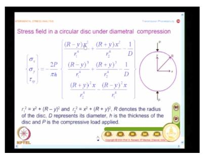
And in the last class, we saw the stress field for the disc under diametral compression and I have sigma x, sigma y and tau xy and these are the expressions we have also noted down earlier and we take the center of the disc as the origin and r is the radius and what I said in the last class was to find out from these expressions, the value of sigma 1 - sigma 2. In fact, what we want is, we want to see principal-stress difference.
