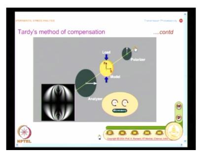
I have a plane polariscope because I have to go to a plane polariscope and then do it. I have the source of light, then I have the polarizer, I have the model and this is what I said, at the point of interest, the reference axis itself is the base reference axis for the final circular polariscope also. In this case, the point is selected as a center of the disc, the horizontal and vertical axis themselves are principal-stress directions.
