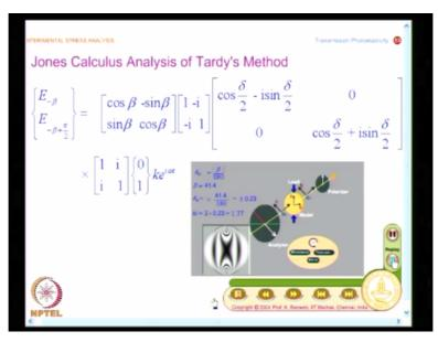
So what I am going to do, I want to find out this. So, I have what is a light that is coming out of the polarizer and then after the polarizer, I have a first quarter-wave plate, I have the model, I have the second quarter-wave plate, then I have the analyzer. Here, I also bring in the analyzer and I also made one more statement when a fringe passes through the point of interest, we are essentially saying intensity goes to 0.
