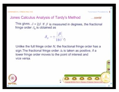
What we have seen is, we get delta = 2 beta and since beta is usually measured in degrees which is very convenient. I get the fractional fringe order as beta/180 degrees and I do not attach the sign. The sign has to be attached based on whether the higher fringe has moved to the point of interest or lower fringe order has moved to the point of interest and this has made conventional analysis very simply.
