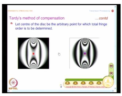
There is a particular reason behind it because the next topic we are going to discuss is how to find out material stress fringe value f sigma? And I would use circular disc under diametral compression as the basic model to be used for finding out f sigma and we will use Tardy's method of compensation to find out the fringe order accurately and what we are going to look at we are going to look at the center of the disc.
