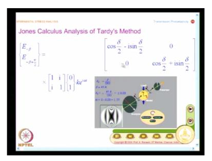
Now, you have the second quarter-wave plate and what is the difference between the first quarter-wave plate and second quarter-wave plate? I have not written 1/root 2 here, because I will write it finally for both the quarter wave plates product of 1/root 2 as 1/2. So, now I will write the second quarter-wave plate that is nothing but 1 - i - i 1 and I also put the rotation matrix for me to find out the component of light vector along the analyzer axis.
