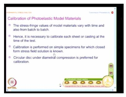
So, you need to calibrate each sheet or casting at the time of the test and what is the thumb rule? When I have to do this, my focus is on finding out f sigma. So, I need to do it on a model for which closed form stress field solution is known because I should conduct the experiment as accurately as possible. So that, I follow all the restrictions on loading and I find out what is the fringe order at the point of interest.
