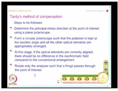
Your interest is only to find out fringe order N, but you also have to find out theta. The second step is I have to form a circular polariscope such that the polarizer is kept at the isoclinic angle and all the other optical elements are appropriately arranged and if you do not align the elements properly, there would be distortion in the isochromatic field.
