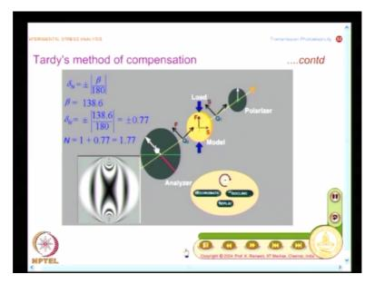
In the second case, a fringe order 1 has moved and occupied. This is the very important information. In fact, this is the advantage in a conventional photoelastic analysis, you get the heuristic information in fixing the sign of the fractional retardation. In fact, this was a very difficult task in digital photoelasticity. Fixing the sign of the fractional fringe order was not a simple task.
