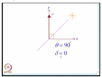
I can say that theta = 90 degrees and delta = 0. I do not even have to go for a matrix representation. I can simply represent this as a vector. I send only a component of light along the y axis is what my vector should say and that is easily represented by 0, 1 a simple vector like this
