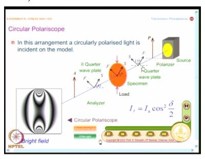
And let us what are all the elements that you have. I have the light source after the light source I put a polarizer. Then I put a quarterwave plate which is oriented at 135 degrees. Then I put a model which is loaded. After the model I put a second quarterwave plate adn this quarterwave plate is kept at 45 degrees then I put a analyzer. so in a circular polariscope I have 2 elements before the model and 2 elements after the model and if you watch it very carefully.
