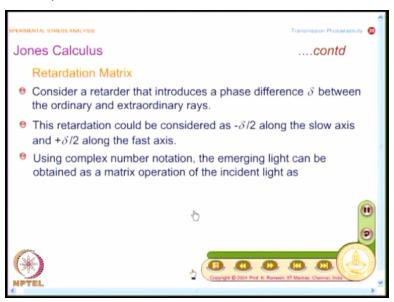
And what we want to do we will consider a retarder that introduces a phase difference delta between the ordinary and extraordinary rays and how we introduce this delta this can be written down in many different ways and I said that retardation could be considered as - delta/2 along the slow axis and + delta/2 along the fast axis. So the idea here is we would like to have a nice matrix representation and we will follow some convention to facilitate.
