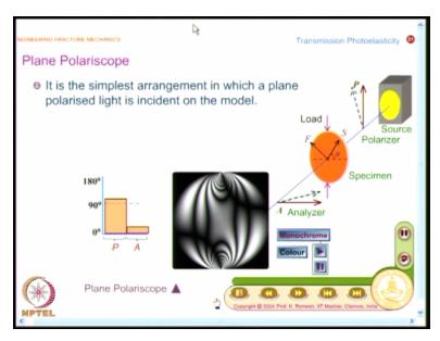
We had a light source, then we put a plane polarizer. Then you had a model which is loaded and you analyzed whatever the light that comes out of the model by an element similar to polarizer but the axis is different, because you do the analysis of exit light ellipse you call this as analyzer and what we saw in general in a plane polariscope you would see 2 fringe contours. One fringe contours move as the polarizer.
