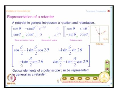
So I have a rotation matrix as light hits the retarder within the retarder it introduces as a retardation and whatever the modification that has been done by the model I want to refer it back to the original reference axis as x, y so I put a reverse rotation matrix, but what I want is I want you to do the matrix multiplication right in the class and when you do this you expand this e power - I delta/2 as cos delta/2 - I sin delta/2 and do the simplification.
