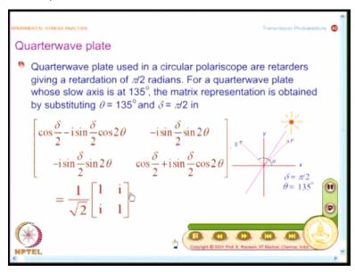
So that is what we will have a look at it and then we have this as quarterwave plate and quaterwave plate used in a circular polariscope are retarders giving a retardation of pi/2 radians. So we know the retardation and we keep the quarterwave plate at appropriate angles. One such angle is 135 degrees. The other angle is you can also keep it at 45 degrees and look at how the retarder is represented.
