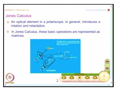
We will have to understand first of all that an optical element in a polariscope in general introduces a rotation and retardation and our interest is you know you want to have this as matrix operators with that the analysis becomes lot more simpler. So this is what we want to look at. The basic operations are represented as matrices and I said in one of the earlier classes when we introduced this.
