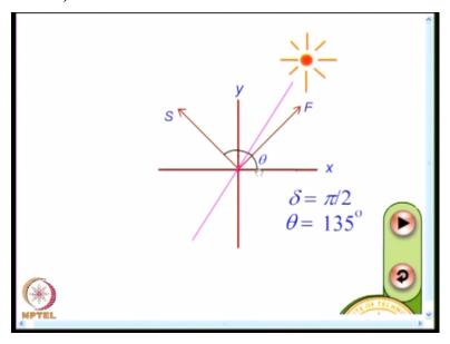
So what I have here is I have the reference axis as x and y. I have a quarterwave plate with slow axis adn when I show theta I show the reference from the horizontal to the slow axis. Theta is the angle of the slow axis and fast axis represented here. So when I have a quarterwave plate oriented at 135 degrees I write delta = pi/2, theta = 135 degrees. On the other hand, if I put theta = 45 I would get a different answer.
