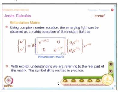
So what I have here is I have u prime, v prime which is = we take the real part of e power - I delta/2 0, 0 and e power I delta/2 and why I have e power - I delta/2 here because I understand that this is a slow axis and this is the fast axis. So because I write my retardation matrix with the first element as e power - I delta/2 I should always represent theta referring to slow axis with respect to the horizontal and this is the general light that is impinging on the retarder.
