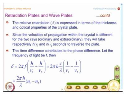
So what we want to do is we want to express the relative retardation in terms of the thickness and optical properties of the crystal plate. So what we want to do is when I say optical property what are the properties I have refractive index n1 and refractive index n2 or you can also classify it as ordinary ray of refractive index and extraordinary ray refractive index that is fixed for a crystal.
