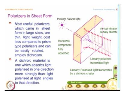
And that is what we have looked at in the last class polarizers in sheet form and what we learnt was within the polarizer sheet the horizontal component is absorbed by the polarizer and for illustration this is shown which large thickness in reality this is very thin and this phenomenon is called dichroism. So a dichroic material is one which absorbs light polarized in one direction more strongly than light polarized at right angle to that direction.
