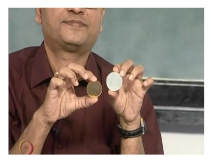
Okay let me go back to my other question that I raised about 3 classes back. I took an aluminium disk and also a Polyurethane disk. I said poly is one of the photoelastic model material and then imagine that I apply a same load. I said what is the nature of the stressors developed because Polyurethane is a plastic which has low angst modules you can visually see the deformation.
