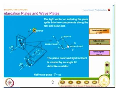
And what happens when I go to a half wave plate. When I go to a half wave plate a simple argument is I will have instead of acos omega t. Suppose I will give only in this there is a retardation this will become acos omega t+ pi so that is nothing, but –acos omega t. So you will have a component here. So you will have the resulting will be in this direction. So plane polarized light which is incident on the model remains plane polarized, but rotated by angle 2 theta very interesting.
