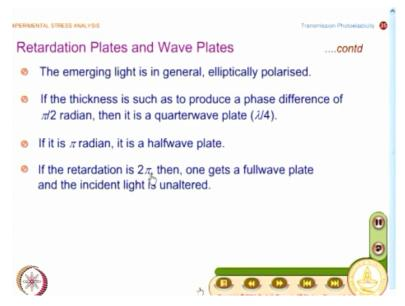
So what you find the first observation is when I have a crystal plate even when I send a linearly polarized light impinging on the crystal plate. The emerging light is in general elliptically polarized. So that is the general observation number one. And if I so adjust the thickness of the plate to produce a phase difference of pi/2 radian then I call that as a quarter wave plate. It is also labeled as lambda/full plates.
