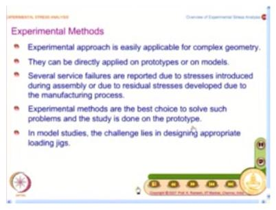
Once you come to experiments, what do you see. Very similar to numerical methods, experimental method is applicable for complex geometry, absolutely no problem and once you come to experiment you will also have to look at 2 different things, am I working on a model or am I working on a prototype. So, you can do the experimental approach on prototypes or on models. Another area where experiment methods are the ideal choice is in the area where you have assembly stresses or residual stresses.
