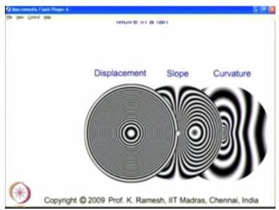
What you find here is for a circular plate clamped at the boundary with a central load you get the displacement and you can also have the slope, you can also get curvature. But will I had appreciated here is for each of these information you need to use a specific optical arrangement. You do not get them in one shot but you have to have effort to do that and you see on these 2 corners show that you need to use physics in applying experimental techniques.
