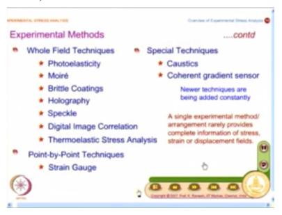
When you look whole field techniques, one of the very popular and widely used experimental method is technique of photoelasticity and we would see later what these experimental techniques give directly the information, what information it can give directly. Essentially, photoelasticity gives sigma 1-sigma 2 contours and you have Moire that essentially gives displacement and you have brittle coatings that gives direction of principle stress.
