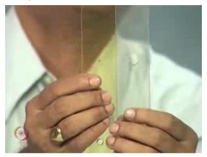
On the other hand, if I take a model with a slightly larger hole, then this solution is no longer valid. I have the same width. The width is same. In one case, there is very small hole. In another case, the hole is about 10 to 12 mm and this is comparable to the width. So, this becomes a finite body problem. So, when I go to theory of elasticity where I am to idealise. I look at a situation where I remove the restriction on displacements and I evaluate displacement as part of the solution.
