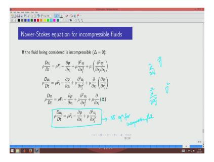
So, here is basically the Navier Stokes equation for incompressible fluid and this operator  $\frac{\partial^2}{\partial x_j^2}$  is nothing but the laplacian operator. So, you could actually write that also and this operator is nothing, but the gradient operator. So, you could actually now write the Navier Stokes equation for an incompressible fluid using the vectorial operators as well. That is what we do here.
