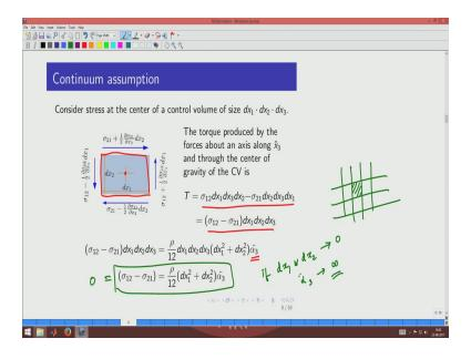
So, here I want to argue that stressed tensor is symmetric tensor. So, you could just simply state that stress is defined for continuum and therefore, it must be a symmetric tensor, but we can see why. So, let us take a control volume that is drawn here. So, the control volume is drawn here in this manner, and at this point we inspect how the forces are going to act if they
