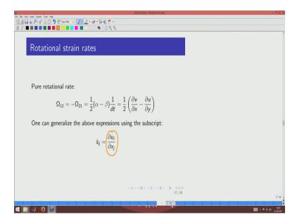
And similarly the rotation also can be written the different of those angles that gives the rotation. So, you could see that this quantity is very generic quantity it is a strain rate tensor and it has basically the diagonal terms off diagonal terms and they seem to have some meaning.
