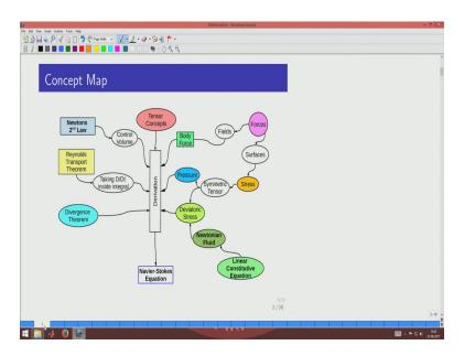
So, the concept map for the derivation of Navier Stokes equation is given here. The starting point for the Navier Stokes equation is nothing, but the Newtons second law the conservation
