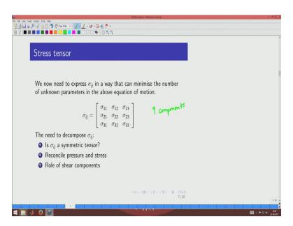
So, what you are going to do is  $\sigma$  is basically a stress tensor and if you expand it because it is a tensor of order two you will have it as 9 components. So, you could see here 9 components
