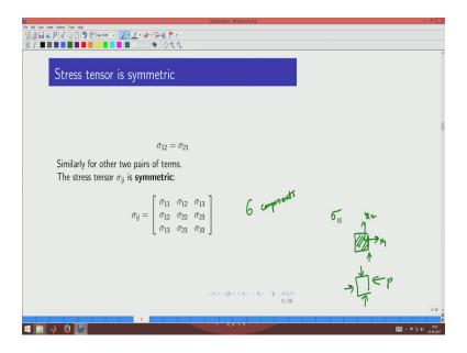
So, we say that if  $\sigma$  is a symmetric tensor we now have written here  $\sigma_{12}$   $\sigma_{13}$  both ways and  $\sigma_{23}$ , both ways which means that we now have 6 components that are to be determined. So, from 9 we have got 6. So, there is some progress.
