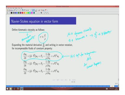
So, we use the vectorial operators and we have the gradient here, we have the see the left hand side as  $\frac{d}{dt}$  the material derivative we are expanding the material derivative on the left hand side and on the right hand side we have got the gradient operators and the Laplacian operators we use. So, you could see that this now becomes the in vectorial notation the Navier Stokes equation for incompressible fluid.
