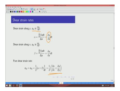
So, the shear strain is defined in this manner  $\frac{PQ_y}{AB}$  and then if you then look at the locations and derive you can see that the shear strain rate is given by this you can see the cross terms v and x up in two different directions are coming together. So, shear strain is coming like that. And then the pure shear strain is written as an average of those two angles and then you see that this is how it is coming up.
