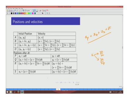
So, what we do is basically ABCD the locations we write the coordinates  $x_0$   $y_0$  and the velocities are u and v. And in general there are these gradients that are present, so u has the gradient in both you know x direction as well as in y direction. So, let us see how the velocities are specified.
