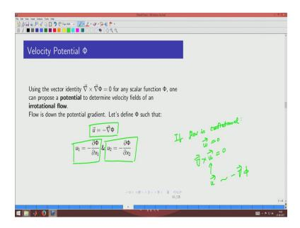
So, the reason why we have actually come up with this particular type of flow is because it allows us to define another quantity which we call as velocity potential. So, that we can actually generate the velocity components for a very specific 2D flow situations. So, we call that as basically velocity potential in the following manner.
