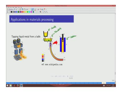
So, here are some real life situations encountered in metallurgical industry where these elementary planar flows can be used. For example, here this is what we call as a Ladle and this is what is called as a Tundish and the process that we are seeing here is continuous casting process and this is the Caster. So, liquid is coming into the caster and then it is becoming solid. So, by the time it comes out everything is ready here which means which is fully solid, the yellow is the liquid metal.
