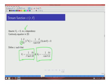
And we could also do that in spherical coordinate system and the difference between spherical and cylindrical will be evident here. So, watch out the power of r. So, you could see that here it is  $\frac{1}{r}$  and here just  $\frac{1}{r^2}$ .
