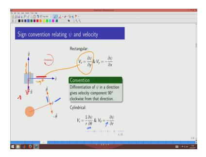
But there is a convention by which we define and that is the convention is what is being introduced. The convention is as follows the derivative of  $\psi$  if you take along 1 direction then 90° away in clockwise is the velocity component being given. So, which means that if you look at this first expression you can see that  $\frac{\partial \psi}{\partial y}$  is being taken in this direction and then 90° away is this direction which is x which means that is what is being given as a component.
