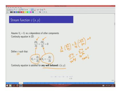
So, we are now going to reduce the number of unknowns in a 2D field. So, you have basically 2 components of a velocity field. Here we are having them as  $V_x$  and  $V_y$  as the components in 2D, which means that we now have the continuity equation having only 2 terms and that is written here and we can use this equation to reduce the number of unknowns from 2 to 1. So, the way we do it as follows.
