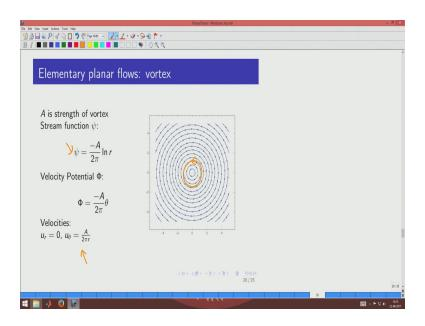
The last one is vortex flow. So, vortex flow as a name indicates should have a rotatory motion of the liquid. So, we can see that vortex flow would look like that, where the liquid is going around and you have basically that as only the  $\theta$  component being present r component is not there. And you can already see that the magnitude of the velocity should go down as  $\frac{1}{r}$  cylindrical coordinate system and that is also satisfied. So, you could plot the contours of  $\psi$
