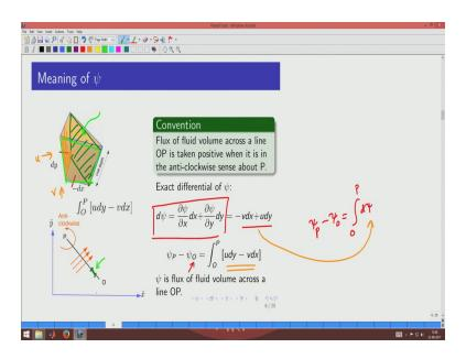
Now, what is the meaning of this function stream function we have mentioned that it is useful it will definitely reduce a number of components from 2 to 1, but then does it have any sense in the what we can actually call it as. So, we have that being defined here. So, consider a small volume element and remember that we are using it for 2D flows. So, the area element in 2D will become a line element. So, we want to consider a line element as follows. So, I take a line elements like this.
