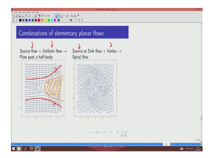
Now, the application of elementary flow fields is to describe situations that are closed to real life situation and be able to combine the elementary flow fields to arrive at a flow field that looks quite realistic. So, you could already see that in this case flow past the half bodies, where is that half body? You could think that the half body is like that. So, you have, how does the flow happen around that, that is what actually is now being shown.
