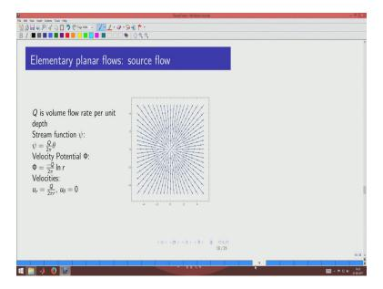
So, the source flow is the exact opposite of sink flow. Here basically the directions of the arrows are reversed and you could see that it can be given by the function that is just with a minus sign. So, you could also see from here the velocity components are just plus of  $\frac{Q}{2r}$ . So, the quantity Q in both the sink flow and source flow basically indicate the volume flow rate per unit depth the z direction and that can be used to calibrate the velocity components in the r direction.
