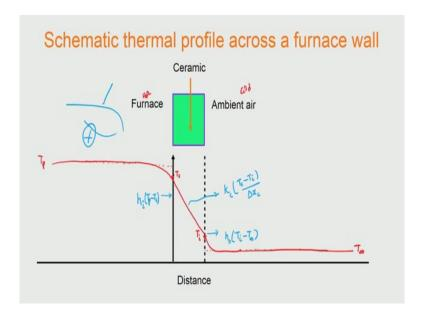
So, let us a for moment we ignore this particular aspect, we do not want to talk about the air gap at all, and want to only draw the schematic temperature profiles across the furnace wall.
