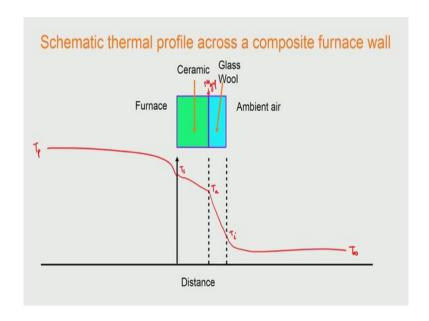
So, we increase the layers and see how this should be drawn when you have a composite wall, and then while drawing that we already know are practicing. So, we realize that the ceramic is having a better conductivity compared to the glass wool. So, we say that the glass wool should withstand a large gradient and then the ceramic should withstand is smaller amount of gradient, and then we see that this has to go something like that and this has to go something like that.
