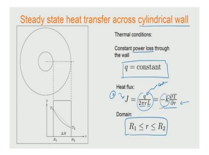
So, we can then look at the same thing in other coordinate systems as well. So, we take up this cylindrical wall now. And in the case of cylindrical wall we again look at the same problem, it is the power loss which is given as a constant and then we already saw that the power loss is q, and the flux is then given by q/area.
