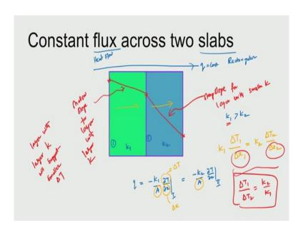
So, for that what we do is, first let us look at how to draw the situation when there is a constant flux across the slabs. So, we take rectangular case, which means that constant flux and constant heat flow are same, and we say that, that is basically q which is going out in this direction and that is constant ok. Now, what we do is that, let us assume that the first case  $k_1$  is the thermal conductivity.
