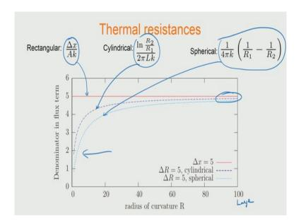
So, here we now write and summarize what are the thermal resistance that we came across in the case of rectangular system. We got the thermal resistances  $\Delta x/Ak$  in the case of cylindrical, we got it as  $\ln (R_2/R_1)/2 \pi Lk$ , and in the case of spherical system we see it as  $1/4 \pi k$  into the difference of the inverses of the radii.
