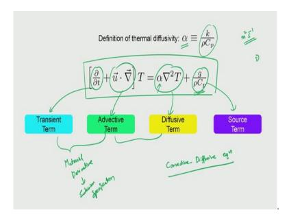
So, we can then take it to the right hand side and write it as follows. So, when you take to the right hand side  $k/\rho C_p$  comes, and  $k/\rho C_p$  can then be called as the thermal diffusivity, which has the units  $m^2/s$ , and we already saw some quantity of this nature and v in mass transfer also, earlier the momentum transfer we look at what is called as the momentum diffusivity and that is basically v kinematic viscosity and that has also the same units ok.
