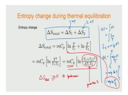
So, you write the entropy change for the entire body in this manner. So, you say that the entropy change for the first body is  $\Delta S_1$  and for the second body is  $\Delta S_2$ . This is going from  $T_1$  to  $\acute{T}$ , this is going from  $T_2$  to  $\acute{T}$  and you could write the  $\Delta S$  is basically  $\int dS$  and that we write as  $\delta q/T$  and we already know that  $\delta q$  is given by for example,  $mC_p \times dT$ .
