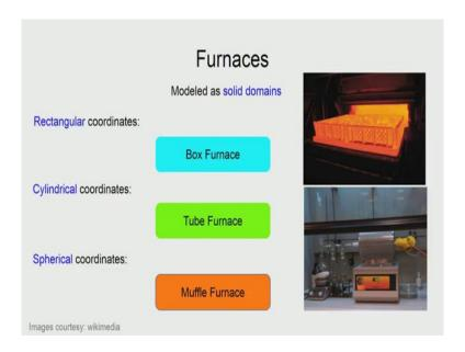
Now, here is where actually all these three coordinate systems are going to be useful metallurgical scenarios. So, in metallurgy we have heat treatment; that is happening for you know many components, and that is one problem where the heat transfer is directly used in a solid state, and so we have basically the furnaces where the heat treatment is being done.
