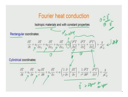
So, the Fourier heat conduction we now then expand. So, what we do is this equation we expand. So, we expand these terms in different coordinate system. So, for rectangle coordinate system we expand the advective term, we can immediately see that this can then be expanded here, and  $\nabla^2 T$  can be expanded here. So, this is the first and this is the second, first operator and second operator.
