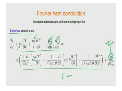
And for a spherical coordinate system. So, the equation looks like this. So, you have got  $u_r u_\theta$  and  $u_\phi$  coming in, and the Laplacian term for spherical coordinate system is looking like this. Notice that the power of r is different from the cylindrical coordinate system in cylindrical it is r and here for a spherical it is  $r^2$  that is coming in ok. So, other than that you can actually look up these from handbook and substitute directly ok.
