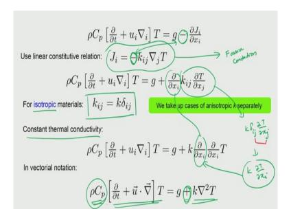
Now, the flux is then expanded, and we expand the flux in this manner, where we basically already have talked about it, it is basically the Fourier conduction, Fourier heat conduction equation, the flux is equal to  $-k \times \Delta T$ , and the k for example, here is a tensor of order two, then we want to make a simplification that for isotropic materials we want to consider it as an isotropic tensor and therefore, we can write it as  $k \times \Delta_{ij}$ .
