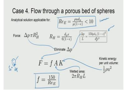
So, the expression for porous medium which is made of a bed of spheres is actually identical to the porous medium you have seen earlier; except further to the  $S_o$  is taken as  $6/d_p$ ; though the reason being that when you are assume that the spheres are all touching at the point contact. And then you can directly get the wetted area per unit volume of the solid analytically and that comes as a  $6/d_p$ ; where  $d_p$  is the diameter of the spherical particle that is consisting in the bed.
