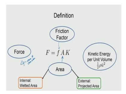
See the definition is as follows; friction factor is this quantity f that we have written here and it is defined as the expression here F capital F which is a force is equal to small  $f \times \text{ area } A \times K$ ; which is the kinetic energy per unit volume. So, if you see this K and if you multiply with the volume then you will get the kinetic energy half  $mv^2$ .
