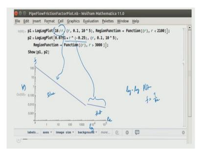
So, you notice here that it is log and the log plot. So, remember that it is always made a log log plot and the log log plot of a function that looks like f is equal to something by Re, you would be naturally have a negative slope of one which is 45 degrees in the negative way, which you can already see that is visible here.
