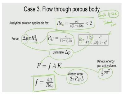
So, that is how you got the analytical solution here which we gave a name Blake Kozeny equation and the bundle of tubes would mean that it is actually internal flow; so, this is important. The model that we have chosen is that it is an internal flow which means that even though the porous body is made of spheres, where actually the liquid is going outside of the sphere; it is still not treated as an external flow, it is treated as an internal flow because of the void is being modelled as a pipe.
