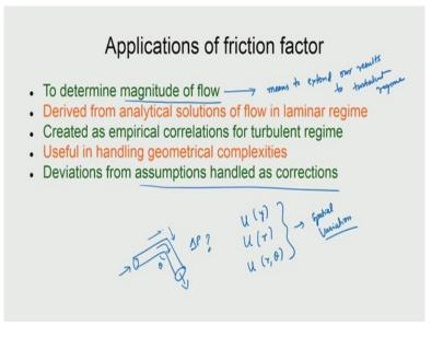
So some of the applications of friction factor why do we need this concept at all? So, we have already seen that we have the analytical solution for the velocity. So, if you have u and you already have u as a function of r, u as a function of r and  $\theta$ , u as a function of y and so, on.
