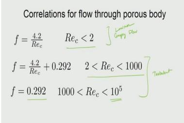
So, how does this expression then change when we go to other regimes? So, it is again seen here that friction factor is defined for less than 2 Reynolds number. But when you go to turbulent regimes these are all turbulent regimes; so, this is basically creeping flow regime, so for turbulent creeping flow or laminar regimes.
