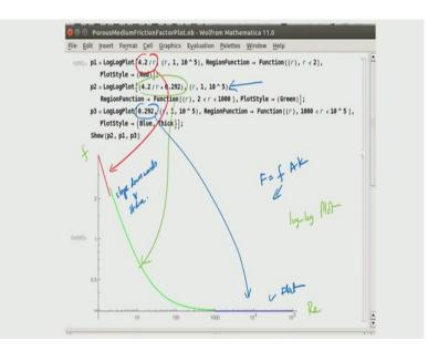
And when we plot these using the mathematical notebook, we will see that the three expressions are appearing to be the same. So, the log log plot has a the friction factor as a function of Reynolds number is appearing to be straight line drooping downwards on the left hand side for the low Reynolds number and a flat region on the right hand side for the turbulent regime.
