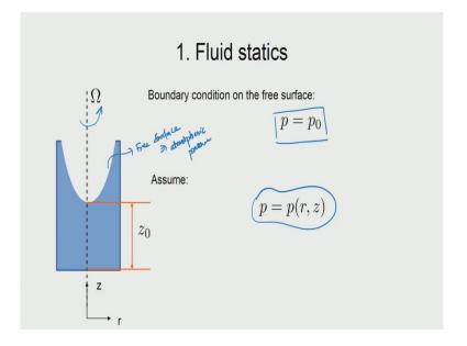
So, first problem is about statics problem namely the situation where we are only looking at how the pressure would change as a function of distance. So, here is a situation where you have a container of liquid which is made to rotate about its own axis. So, this is the rotation that is happening and because of this we expect normally that the liquid will be pushed away from the centre so it would climb up the wall little bit and it would take the free surface would take a shape.
