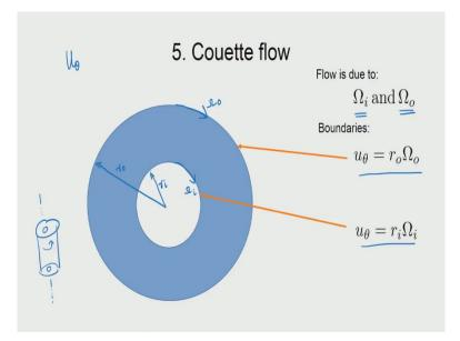
Now, we take the last component of the velocity the cylindrical coordinate system named the  $u_{\theta}$  now  $u_{\theta}$  of in this particular problem is actually called as the solution for the Couette flow.
