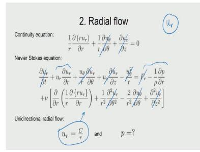
So, the radial component is being taken. So, radial velocity component is  $u_r$  and the continuity equation needs to be satisfied and also the Navier-Stokes equation. So, we saw that if you look at only the continuity equation we already can guess what kind of forms are
