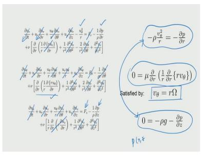
Now, this equations are going to be very trivial because we do not have velocity components except in the  $\theta$  direction, because r velocity is not there, wherever  $u_r$  is there those components will be all going off. So, I strike off all those and we also know that we have chosen the axisymmetric situations. So, we strike that off also and there is no body force term
