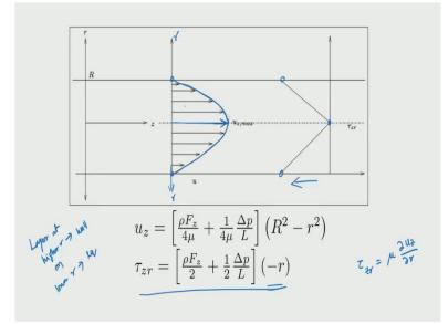
Now, when we plot this parabola it would look like here. So, this is the plot we are trying to show, which means that in the tube at this centre is the maximum velocity and at the walls it is 0 velocity and the slope at the centre will be 0 and the parabolic is a nature of the velocity as a function of r in the tube.
