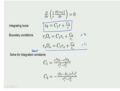
So, there are two integrate integration constant  $C_1$  and  $C_2$  and when we substitute the boundary conditions we can determine. So, the inner wall boundary and outer wall boundary conditions are listed here. So, what we do is at the first one if you multiply with  $r_0$  the first second equation if you multiply with  $r_i$  and then if you subtract then you could see that you would eliminate the terms and then start to see the solutions.
