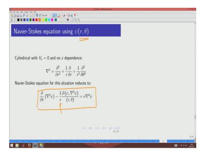
So, if you take cylindrical coordinate system for example,  $r_{\theta}$ ,  $r_{\theta}$  that is the planar flow in a cylindrical coordinate system the z direction velocity is not playing the role then it looks the same way. Only thing is that there is a additional term that is coming in because of the curvilinear coordinate system that we have used, but the nature of the form is the same and in case you are looking at axis symmetry.
