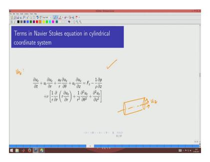
So, you can see that Navier Stokes equations are basically sets of three equations in the case of rectangular coordinate system all the three terms look same whereas, in the cylindrical and spherical coordinate system they do have small variations here.
