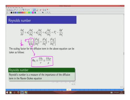
So, we define Reynolds number like that. So, the inverse of this quantity is defined as the Reynolds number. So, you could see that the Reynolds number is naturally coming out of the Navier Stokes equation as a scaling factor coming in front of the diffusive term and the units are wiped off because the non-dimensional is done for all the terms.
