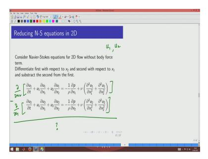
So, now, what we have done in the session on planar flows is that if you have 2D flow you have got two components of velocity and if you want to reduce the number of unknowns to just 1, then we have come up with stream function which can generate those two components and then we saw that the equation just comes down by 1.
