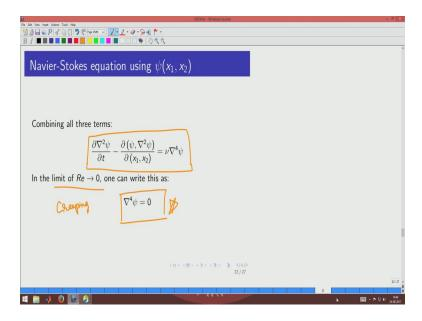
So, you can see that this particular equation we then you know for stream function and we have only one equation. Now if you solve this equation and get the solution for  $\psi$  and then differentiate  $\psi$  with respect to  $x_1$  and  $x_2$  then you have got the velocity components in 2D. So, with one equation you have got two velocity distributions that are available. So, that is the simplification we were seeking when we introduced the concept of stream function at all.
