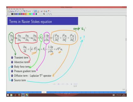
Now, we now being our attention to the different terms of the Navier Stokes equation we want to call different terms by names, so that later on when we solve some problem we want to see which terms can be knocked off and we can make a simpler case of Navier Stokes equation to obtain the exact solutions of that for a given problem.
