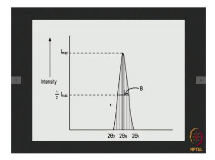
So, it has a measurable breath at half the maximum intensity. So, whenever we have a line profile, we measure the breadth of the line profile at half the maximum intensity. So,
