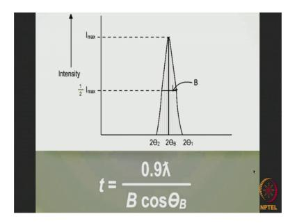
So, this is the situation if this is the breadth of the line profile we can find out t is equal to 0.9 lambda by B cosine theta be this is the well known Scherrer equation.
