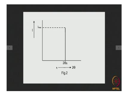
Now when we have the Bragg law perfectly satisfied, then what we expect we would expect that all the diffracted intensity will be concentrated at 2 theta B where theta B is the Bragg angle. So, this should be the shape of the diffraction line profile for when Bragg's law is perfectly satisfied, but what we observe in practice in practice you find a diffraction line has this kind of a profile.
