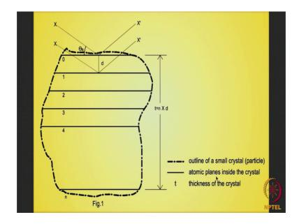
So, this is what I have already explained. So, this is say the outline of the crystal we are considering and there are planes marked as 0, 1, 2, 3, 4, etcetera up to n. So, the thickness of the crystal t we can write as n into d where d is the inter-planar this terms. So, this is the situation t is equal to n into d. Now when perfect Bragg law is satisfied for
