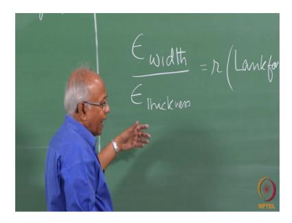
Now this ratio is known as r it is call the Lankford parameter, so Lankford parameter. So, in order that the steel can be deep drawn it is essential that this value is much higher than this value that will ensure. That when we draw the steel you know when it will spread in
