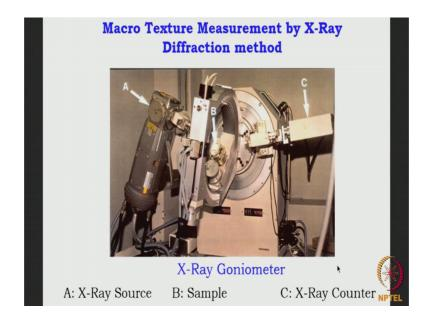
As I said macro texture measurement is normally carried out by X-ray diffraction. Now this is an X-ray diffraction unit with what is known as X-ray texture goniometer. So, here this is the X-ray source and you have got your specimen over here, and you have got the X-ray counter to measure the diffracted radiation in this direction.
