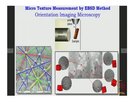
Now if you look at the electron backscattered diffraction pattern, they look very similar to the kikuchi patterns which are obtained from rather thick specimens in a transmission electron microscope. And from the kikuchi pattern it is possible to accurately determine the orientation.
