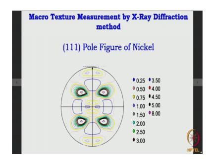
So, this is the pole figure of recrystallized nickel, this is the rolling direction, this is the transverse direction and this is the normal direction. So, all these different colours talk about the densities of the poles over here in terms of random.
