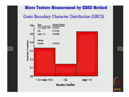
So, what is the fraction of grain boundaries? Which are the low angle boundaries? What are the high angle boundaries? And the c s l boundaries all this information can be obtained from this orientation.
