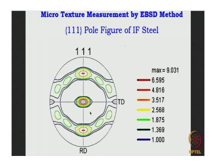
Now, this is the 1 1 1 pole figure of an interstitial free steel which was measured by the EBSD method and this is the ODF of the same steel again measured with the EBSD method.
