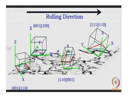
And this is the rolling direction. Now say we consider the grain over here. Now we have drawn the unit cell for the grain in an enlarged manner. So, this is a unit cell of the grain and what is fine that this top plane of the unit cell which is nothing but the 0 0 1 plane is parallel to the rolling plane, is parallel to the rolling plane. Not only that this particular direction of the unit cell which is nothing but the 1 0 0 direction is parallel to the rolling direction.
