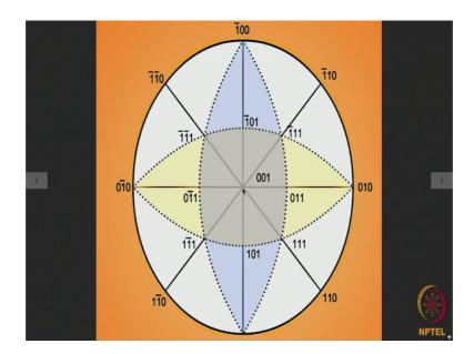
For example, this pole is 0 0 1, this pole is 0 1 0, this is 0 bar 1 0, this is bar 1 0 0 and this is 1 0 0.
