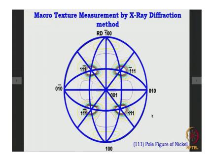
Once we do that you see this is what the situation looks like. So, the blue coloured diagram is the 0 0 1 standard stereographic projection. And below this we have got the pole figure where the 1 1 1 poles have been plotted.
