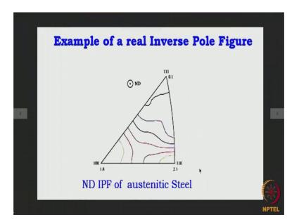
Now example of a real inverse pole figure is giving here. So, this is the normal direction inverse pole figure of austenitic steel. So, here this is the normal direction as important
