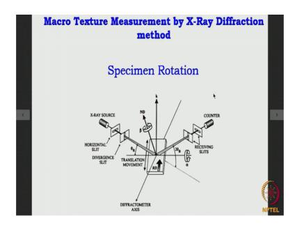
Now the specimen which is put in the texture goniometer is not stationary. In fact, when you have the X-ray beam falling on the specimen as is done you know for normal X-ray diffraction work. The X-rays are incident over a very small area of the sample, you see the small area need not cover many of the grains in the sample.
