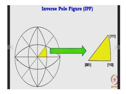
Now let us talk about this second type of the second method of representation of texture. It is called the inverse pole figure method, it is called the inverse pole figure method; if we go back a little bit if you remember the standard 0 0 1 stereographic projection.
