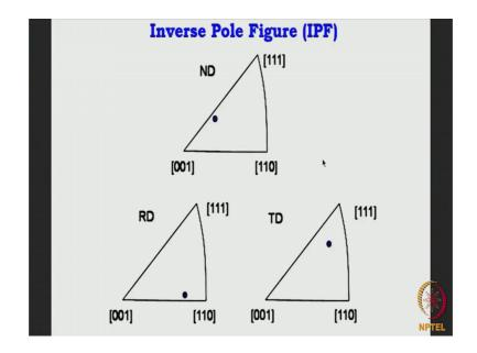
Say for example, we talk about a sheet material we talk about one grain and say the normal direction. What is the normal direction? We plot the location of the normal direction by a point over here.
