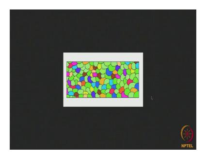
You see that here again a particular grain orientation is denoted by a particular colour. Say for example, this blue denotes a particular orientation of the grains and you can see that not one, but many of the grains have got this blue orientation; that means, many of the grains have got this particular orientation. Again the heavy green colour this green colour is denotes a particular orientation and you can see that many of the grains have got this particular orientation.
