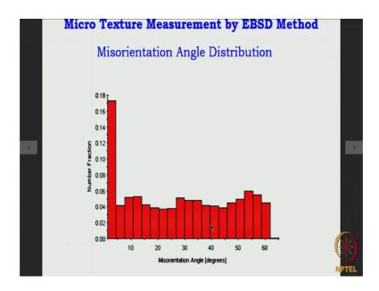
Imaging microscopy it can also a lot of information about how the misorientation angle distribution takes place in a particular area amongst the different grains.
