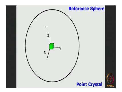
Say for example we are dealing with a cubic material the simplest material and this is the small very small cubic crystal. It is so very small but you can consider it as a single point.
