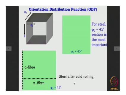
For still engineers the most important section of the orientation space is it phi 2 45 degrees section.
