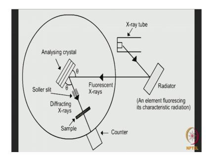
Here, from the X-ray tube the primary X-ray beam is allowed to fall on a radiator. Radiator is nothing but an element which fluoresces its characteristic radiation by the impact of the primary X-ray beam.
