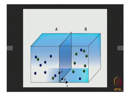
Say for example, we have got 2 metals A and B join together over here and this diffusion couple if it is kept at a sufficiently high temperature for quite some time what will find that atoms of A will move over to B they will diffuse to be similarly atoms of B will diffuse and move over to A. So, when a steady state condition will be reached we should
