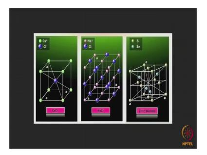
So, there are some examples of compound crystals here it is cesium chloride. So, the chlorine ion is at the center and cesium ions are at the corners of a cubic unit cell. Now this is a sodium chloride crystal, the locations of sodium and chlorine are shown here this is a zinc blende system or zinc sulfide, the sulphur and zinc atom the positions are given here, now I will show it a little bit more detail now.
