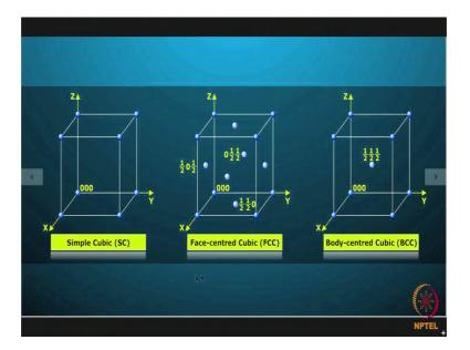
And the third one is the body centred cubic or BCC. Now you will remember that in simple cubic 8 corner atoms the total contribution to this particular unit cell is 1 atom
