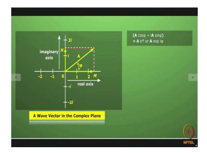
So, how to add up the scattered radiations from all the atoms in the unit cell? So, every scattered wave can be resolved into 2 components one along the real axis and the other along the imaginary axis. For example, if this vector makes a angle phi the real axis then we can write down this vector as a cosine phi plus I A sin phi. So, this quantity can be written either as A e to the power I phi or we can write it as a exponential I phi.
