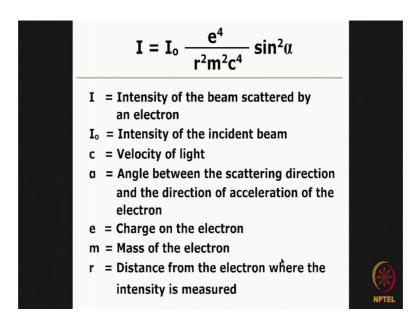
So, here I stands for intensity of the beam scattered by the electron in a direction alpha I 0 is the incident intensity c is the velocity of light alpha is a angle between the scattering direction and the direction of acceleration of the electron or the forward direction e is a charge on the electron m is the mass of the electron and r is the distance from the electron where the intensity is measured; that means, r is this distance.
