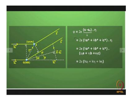
There is going to be a face difference between the 2 and that face difference can be simply written as equal to 2 pi times S minus S 0 by lambda dot r j where r j is this vector connecting the origin to the point to the atom at X. So, this relationship we derived previously. So, this is the face difference between the rays scattered by the atoms at this position and at this position.
