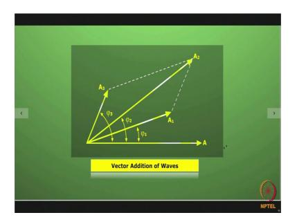
Say for example, we have got say 3 waves one giving by A 1, the second one given by A 2, third one given by A 3. Say with respect to a particular wave A 1 has got a phase difference with it by the amount phi 1 A 2 has got a phase difference with it by the amount phi 2 A 3 has a phase difference with it given by phi 3.
