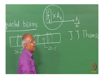
So, in this case f j is the atomic scattering factor of the j-th atom. So, if we multiply it by A e the amplitude scattered by single electron what it gives because, f j the atomic scattering factor is nothing but the amplitude scattered by the j-th atom divided by A e you see f j the atomic scattering factor of the j-th atom is nothing but the amplitude scattered by the j-th atom divided by A e amplitude scattered by single electron. So, if we multiply this with A e.
