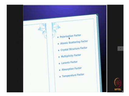
Now, there as various factors which play a role in determining the intensity of a diffraction line: and those have been written down here namely: polarization factor, atomic scattering factor, crystal structure factor, multiplicity factor, Lorentz factor, absorption factor, and temperature factor. Now I will discuss each of these factors separately.
