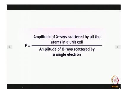
We will now talk about another very important factor and we call it the crystal structure factor we call it the crystal structure factor and denoted by capital F. So, by definition the crystal structure factor is equal to the amplitude of X-rays scattered by all the atoms in a unit cell of a material divided by the amplitude of X-rays scattered by a single electron.
