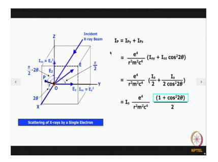
So, the total intensity scattered by the electron at the point p in the x z plane will be equal to I p y plus I p z. So, if we add those 2 up we come to this situation, it will be equal to I 0 e to the power 4 by r square m square c 4 the whole thing multiplied by 1 plus cosine square 2 theta divided by 2.
