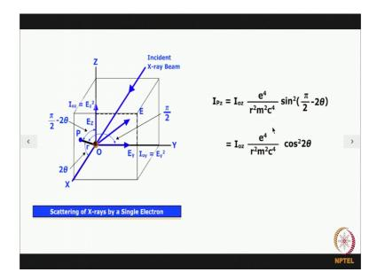
Now what will be the intensity of the scattered radiation by the electron at the point p due to the Z component of the electric vector it will be I o z into e to the power 4 by r square m square c 4 sin square pi by 2 minus 2 theta. So, it will be I o z e to the power 4 by r square m square c 4 the whole thing into sin square 2 theta.
