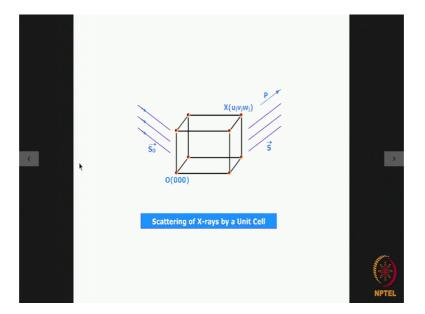
Say for example, this is a unit cell of a material and say a beam of X-rays is incident in this direction and the beam is designated by a unit vector S 0 as we did previously and say the scattering taking place in this direction we are interested to find out what is the scattered intensity in this direction this is denoted by scattered rays are denoted by the unit vector S.
