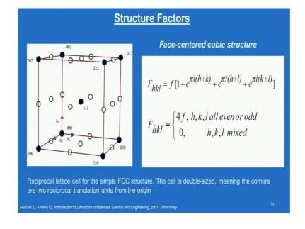
And if you write the expression you have atoms per unit cell. So, you get the 4 terms here. So, 1 plus e pi i h plus k plus e pi i e to the power pi i h plus l plus e to the power pi i into k plus l. So, the rule is f h k l is equal to 4 f where h k l all even or add and the intensity will become our structure factor will become 0 when h k l are mixed.
