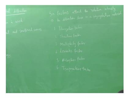
There are 6 factors. So, there are 6 factors that will affect the relative intensity of the diffraction lines in a poly crystal material one is a polarization factor which we have already seen it you know you have some idea about what is polarization factor.
