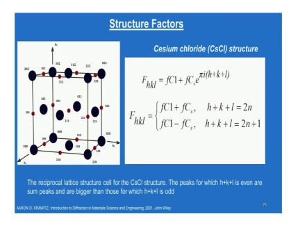
Now we will see some interesting examples a caesium chloride structure where you have a caesium chloride type of structure you can see that it is kind of body centred unit cell has got 2 atoms that is chlorine and caesium atoms per unit cell which is one corner another is in the body centred position, but you can write the expression in terms of the structure factor equation like this and the selection rule is you see f h k l is equal to f C l
