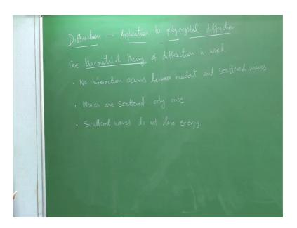
So, before we talk about the intensity of the X-ray peak we should know what is the theory behind it when it being calculations are carried out and so, you see that the kinematical theory is used for calculating the intensity of X-ray and it has got some assumption which is very important. So, I will write down 1 1 3 important assumptions.
