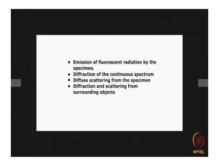
The other source second source is diffraction of the continuous spectrum. You see whenever we use a K alpha radiation you know it is not only K alpha that we use at the same time there will be some amount of the continuous white radiation and a little bit of K beta also because filters cannot efficiently filter the K alpha it is not 100 percent efficient.
