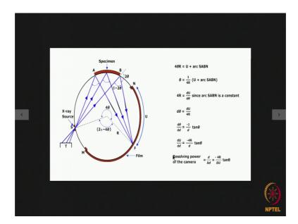
Now if we take a cross section of the Focussing camera as I always said the specimen is an extended one as shown over here. So, we can use a big enough specimen then the x-ray film is placed in this manner the source of x radiation is here and we use a divergent beam of x-rays.
