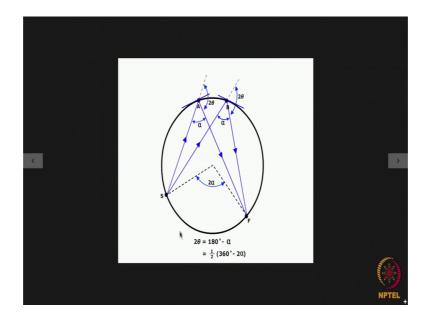
Now in the Focussing method we use an extended sample say we put a sample big enough at the circumference over here. Say these are the two h k l type of planes in the two crystallites in the sample. So, if there is an incident beam over here and it gets diffracted along a particular direction then this angle will be the 2 theta, 2 theta angle is always between the incident and the diffracted direction.
