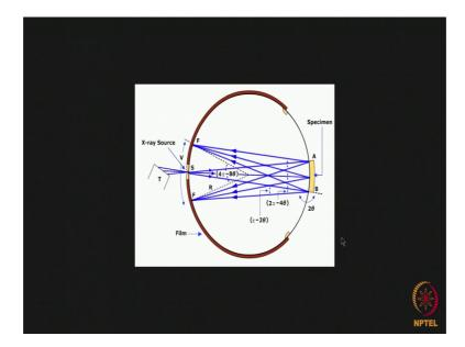
This is the arrangement of the x-ray source, the specimen and the x-ray film in a Focussing camera when we record all the back reflected diffraction beams.
