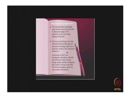
Now, there are two important considerations in this respect the first one is the characteristic radiation which would be used should not be such that it is wavelength is less than the k absorption edge of the specimen why, because this will cause fogging of the film. So, let me repeat what it say the first consideration while choosing.
