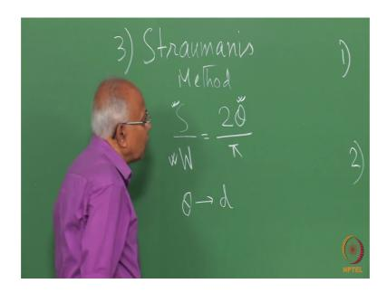
So, there is a third method which is known as the straumanis method. So, what is done here? In this method we have two punch marks two holes corresponding to the regions the collimator and the beam stop. So, the film is plays inside the camera in such a manner that this hole goes over the collimator and this hole goes over the beam stop and the distance between these two holes is known very very accurately from the manufacture of the camera.
