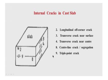
So, again and the slab interior the internal cracks you might see this is a centerline crack or segregation. This is a triple point this is a triple point solidification front moving from here solidification moving from the broad faces, meeting at the you know triple point area. So, this area is very weak. So, you might have crack development at those triple
