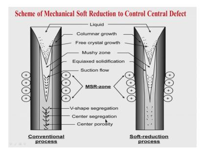
So, also source of cracks I have talked about you know scheme from mechanical soft reduction to control defect at the centre line, I have mentioned two important you know issues here where you put the pressure.
