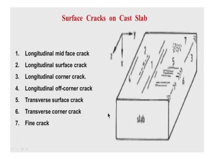
And different orientations longitudinal mid face near the corner at the corner and transverse at the corner all sorts of you know, this is fine cracks without having any typical orientation, but maybe small cracks located at certain areas.
