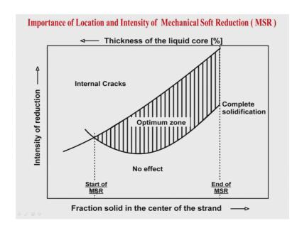
And how much pressure you put this is very important where you put the pressure, you put the pressure near the solidification competition zone and if you put less pressure it will have no effect, if you put more pressure there might be formation of internal cracks. So, the intensity of reduction in centre of pressure has to be some not optimum. So, this is again important issue.
