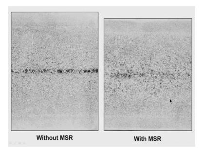
Then how with mechanical soft reduction the intensity of you know central defect, central crack or central segregation is coming down this is just to show.
