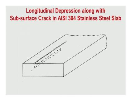
So, this is a slab of AI 304 stainless steel and we have found some depression longitudinal why it is longitudinal because the direction is in the longitudinal direction it was in the direction of the casting.
