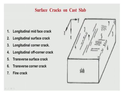
Let us see about this; what is this longitudinal cracks or longitudinal depression at different locations. So, how to take care of this, now I will give you an example of this longitudinal depression how does it look like in actual slab for a stainless steel product we have found out central; central rather a longitudinal depression you see here.
