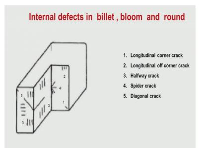
So, you can have this is particularly the central line crack or segregation at the centre of the cast product you can have this. So, it is normally, if it is a long product like you know billet bloom or round or even in slab. So, it is more of longitudinal nature that the central location will have crack as well as segregation. So, which is called central segregation or central crack similar is a case for slab, yeah.
