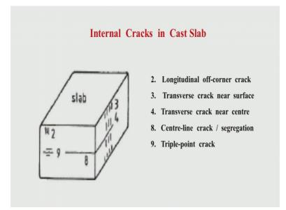
This is the centerline crack or segregation normally some you can had both crack and segregation. So, why the crack is following predominant of the centre because there is
