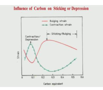
Now, the same behaviour can be shown pictorially based on the distribution of carbon equivalent.
