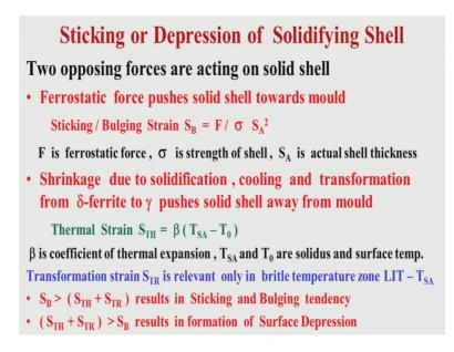
It depends on their value their amplitude which is again a consequence of the real chemistry of the steel. Now how the chemistry is affecting this I have mentioned that chemistry affects the mode of solidification; that means, how solidification is taking place whether initially delta is forming then when delta to gamma is forming when
