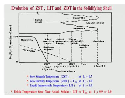
I will give the concept of ZST- I mean zero strength temperature, some people call it NST also that means nil strength temperature. That means, at temperature during casting where the strength is first evolving. The strand initially you have totally liquid and solidification is starting at the meniscus level, as you are going down the continuous caster the solid shell is increasing in thickness, but still there is a liquid. So, it is a strand which is important.
