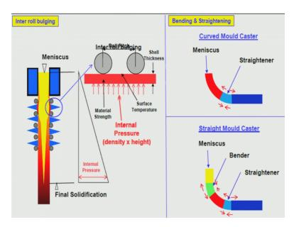
This is the curved mould caster; that means, the mould itself is curved this mould this is the mould, here the mould is indicated as a vertical you know mould.
