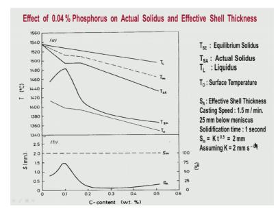
So, I have also mentioned the some values have been shown here some calculated values are shown here for a particular level of phosphorus is 04. So, if 04 percent phosphorus is present in steel, then how this amount of phosphorus effects the actual solidus and the effective shell thickness how is it reduced is shown in this figure.
