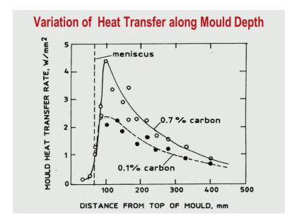
This is another issue which we should know: how the heat transfer varies along the mould depth. This is distance from the top of the mould you know you possibly you know that within the mould.
