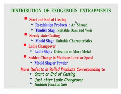
Now, I will try to come to that one by one. Start and end of casting: why there will be mould inclusion, because at those points of time there is a possibility of re-oxidation, because you know you have not you are just putting the Shroud Argon; Shrouding has just started so some amount of re-oxidation is possible. So, these are a distinct possibility at the start and end of casting.
