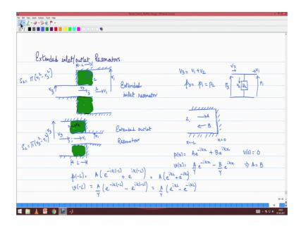
So, the idea is again pretty simple; you will have this is an extended inlet resonator wherein you have an incoming condition which is denoted by 3, the outgoing condition is denoted by 1 and here you have another bypass line which is denoted by 2. And similarly you could have a situation in the of extended outlet resonator which is as follows.
