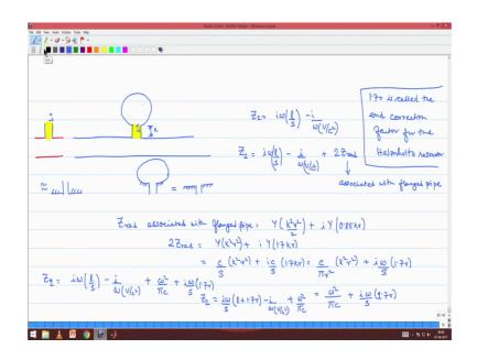
So, we did this Helmholtz Resonator within the acoustic line in the last class. So, there we said that Z 2 is the impedance of the Helmholtz Resonator and that impedance as was calculated earlier is i omega L by S minus i by omega V by C square.
