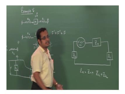
So, the equivalent circuit this time would mean that, you have a source of magnitude F prime plus F double prime. You have a mechanical impedance given by the mass Z m. You have Z s 1 on this side and you have Z s 2 on the other side, that is it right because Z s 2 is basically ending in an open end right. The Z s 2 is this is the only impedance that is there it is ending with a fixed mechanical support which incidentally implies that the circuit has to be left open.
