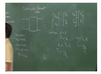
What we will say is that the electrical circuit is going to be represented in this form this is remembered just a representation. Because we realize that it cannot be shunt it cannot be in line. So, therefore, it is a combination possibly of both inline and the shunt, and this is what is called distributed element modelling.
