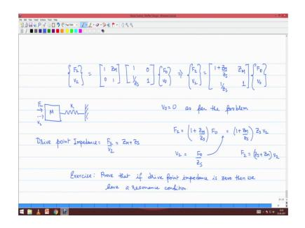
So therefore, it is trivial to find the transfer matrix relating station 2 to station 0 right. That will be the product of the 2 transfer matrices, which are given as 1 Z m 0 1 1 1 by Z s 0 1. And if you multiply them what we get is the following F 2 V 2 is given by 1 plus Z m by Z s. Then we will have Z m, and we will have 1 by Z s and finally, we will have 1, F 1 V 1 sorry, F 0 V 0.
