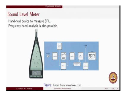
So, I will come back to that question in bit of a time, but before that let us talk about sound level meter. So, in comparison to microphone which is like a real the sophisticated instruments in order to diagnose our (Refer Time: 26:56) related problems the acoustic related problems, sound level meter is a handy device. In fact, our noise police man will have only this sound level meter.
