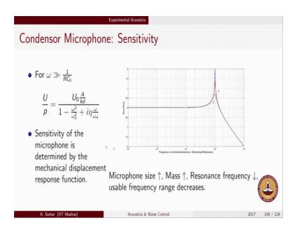
And that clearly shows that the sensitivity remains flat, but provided that the frequency range under consideration is like 0.3 maybe 0.4 times of it is of the mechanical resonance.
