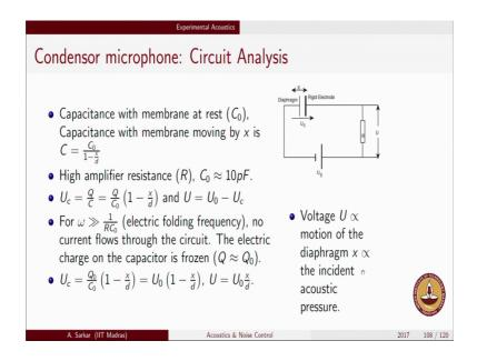
So, let us look at the electrical circuit now as I said to mention to measure this capacitance change it has to be polarized you have you must have a dc source which puts up an initial voltage towards this parallel plate capacitor because if you do not have any initial voltage there is no charge. So, does not work like a capacitor if there is no voltage this no current or charge that will be coming out.
