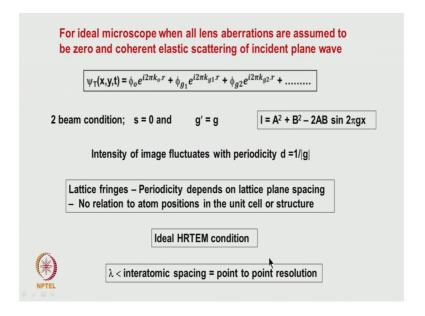
Then what we did essentially was that we try to find out at any point on that image, what is going to be the contribution from the various beams. That is the beams which I have scattered that is from the sampled as the beam enters into the sample, it is getting this is transmitted beam and their beams which are diffracted in different directions D 1 D 2 we want write it all these beams ok they come together and form an image.
