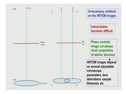
This spread depends upon several adjustable parameters; lens aberrations, sample thickness all and then convergence of the beam there are so many factors independence on ok.
