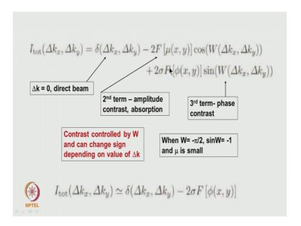
So, as I mentioned now the intensity of the spot if you have to consider it the object function which we have described that has to be that will be modified by this factor that W a to the power of phi W into delta k x minus delta k y this term.
