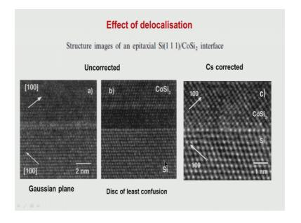
This is another example in which the effect of delocalization; how the delocalization disturbs that atomic resolution contrast are the lattice resolution contrast. This is one where that images as a Gaussian plane and on unconnected one this on a multilayer sample are that silicon with CoSi 2 interface ok.
