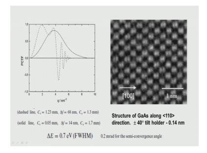
What is being shown is that transfer function for a microscope which is an uncorrected one, and that is where the spherical aberration coefficient Cs is 1.23 m m and this solid length correspond to 1 4 which this spherical aberration has been corrected that is a corrected lens, and for which the Cs turns out to be 0.05 mm we can make out that how drastically testing, then that is defocus also changes that C c value essential remaining the same and the energy of the radiation which is used.
