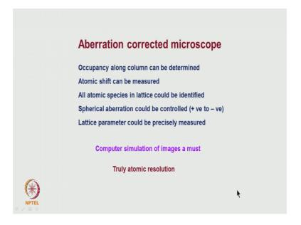
So, what all the advantages occupancy along the column can be determined. Suppose depending upon how much of atoms are going to be along each of the column that information can be and if atoms are shifted from their normal position, what is the shift that of the order of less than 10 picometer that would be measured, then using negative spherical aberration coefficient the transfer function for the different atomic numbers ok.
