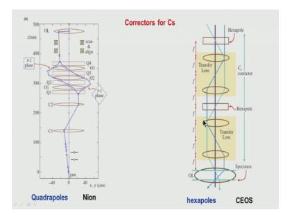
Now that same type of stigmator which are used this could be either quadrapole lenses are this could be a hexapole, there are two types of lens system which has been made for neuron company what they have made it is essentially using some a normal lenses and quadrapole they could make the spherical aberration almost 0, they are same thing which could be done this was that see was Germany this was developed, ok.
