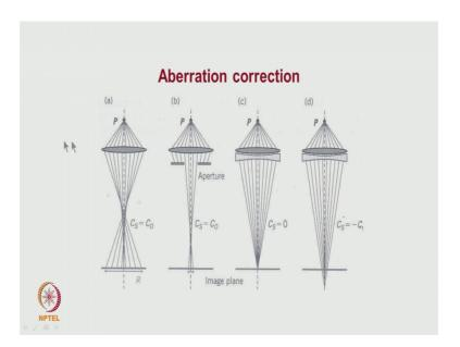
A schematic diagram which I am showing it here is using a convex lens, which has a spherical aberration some value. So, because of this at the Gaussian plane we get some image and then there is a disc of least confusion whether the size of the image reduces. How to reduce the effect of this spherical aberration? We put an aperture so that the of x
