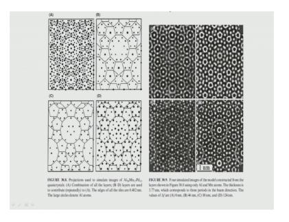
What is beings for a quasi crystal various positions of atoms and various planes is being shown three planes, which are shown and the calculations are done to find out how the end of each one of now them the fourth simulated images for this models are being shown we can make out that this shows the fivefold symmetry.
