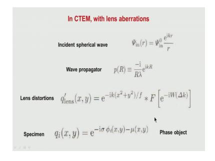
You have a spherical wavelet which is getting emanating from these points from each of this point the spherical wavelets. If we consider that any particular point p here there is going to be a contribution from the various regions of this point from those spherical surface and that is how we can find out what is going to be the amplitude at this particular point when the wave propagates.
