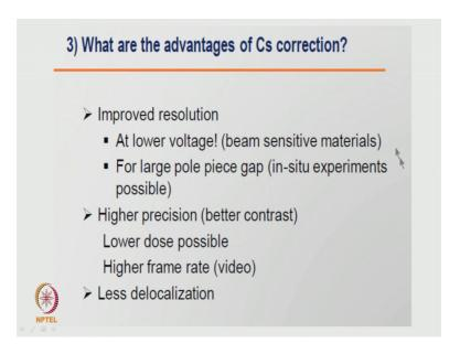
So, what is the advantage of Cs correction? That is Cs essentially is spherical aberration is corrected or not only the spherical aberration can be corrected now the spherical
