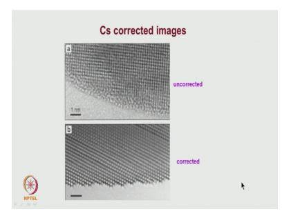
What is the effect of making the deam delocalization? Because edge of it the fresnel fringes appear the effect of these Fresnel fringes essentially going to be that blurring of the image which takes place here ok.
