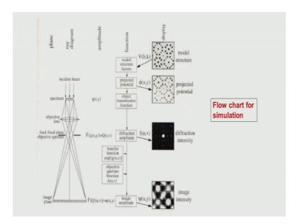
This is exactly what is being shown for a microscopy in this schematic flow chart of that simulation which is normally used, this is the model structure which we use it this is a projected potential for that model structure, ok.
