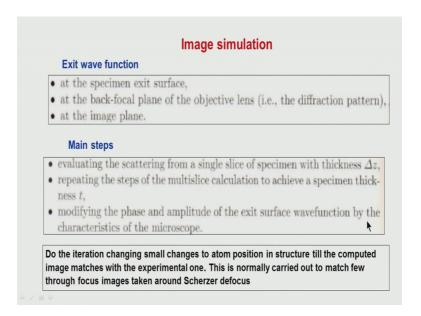
So, in short if you summarize what do you do in image simulation, the first thing which we have to find out is that exit wave function at the back of that sample. Because the beam is a perfect plane wave which is coming into this one and the plane wave passes through that sample and then what is going to be the wave function at the exit one.
