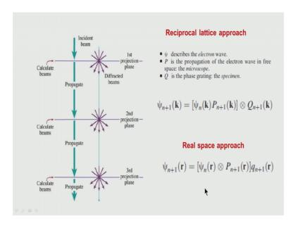
So, as I mentioned earlier that incident beam as it context, it passes through the sample there are many diffracted beams this propagates and the as it reaches here we get the new the wave function is going to be different, the again it propagates this is what we have cal done earlier. So, essentially what happens if that in this case that psi describes the electron wave, P represents the propagation of the electron wave in free space that is in
