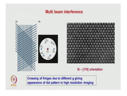
If we use multiple beams then fringes due to each of the beams we will be getting, it actually this fringe space if you look at it the spacing that is that planes on which the maximum or minimum intensity occurs, they are perpendicular to their diffraction vector.
