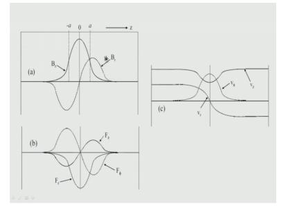
Here is how the forces on electrons as well as the magnetic flux field lengths and how the velocities are affected, this is being shown and in this particular case, one can immediately make out that if we look at it, it looks like a cylindrical geometry like a solenoide.
