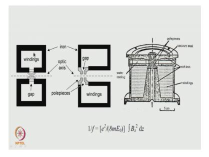
So, this is how these calculations are done. This is what it is being plotted. So, the net effect essentially is that an electron which is deviating from here is brought back to a focus. So, this solenoide acts like a lens. So, this solenoide coil itself can be surrounded with a soft ion piece, so that they capture all and with that we can have lenses with different types of shapes.
