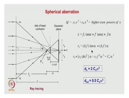
Let us come back to the spherical aberration. What is spherical aberration? The spherical aberration is nothing but when we try to draw the ray diagram for a lens, ok.
