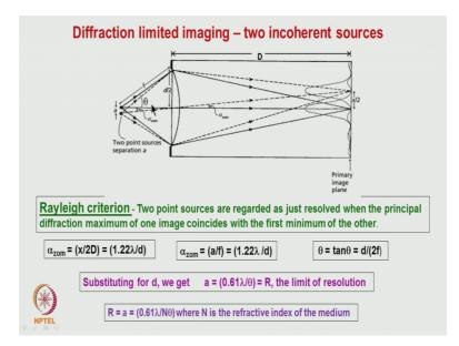
Then, this factor alpha, the angle which submits this turns out to be 1.22 lambda by d, ok where d is the diameter of the aperture. So, if this diffraction limited for what we have considered earlier is for one point source, what is the sort of an image which is formed.
