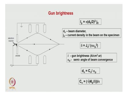
Now, if we take a light source itself if the light source is thermionin source, then what is going to happen is, the electron emission is taking place from a finite area of that sample. So, the current density is one that matters and this also gives rise to some practical limit and the size of the source which we can use it, this size of the source also has an effect on the resolution.
