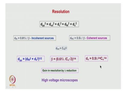
What is the spread which is going to cross for two point which are separated by a finite distance? It is decided by the spherical aberration, chromatic aberration and then due a inherent property of the source, this is Rayleigh criterion and then, another due to a finite size of the source itself. In this we have just taken the square of all the terms are added,
