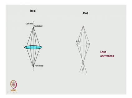
So, if the resolving power of the lens like for example, in the case of an electron microscope which is operating at it 200 kev, the wavelength of the radiation lambda is of the order of 0.0025 nanometer. That means, this is the limit of resolution. So, for an ideal lens all the atoms in the crystal should be resolved, but that is not what it happens. This is because of various lens aberrations which are associated with the lens which we will come to shortly.
