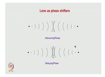
So, this same rate racing itself we can look at it in a different way. Instead of a ray if we consider the light as a way which is propagating, then we can think of from the object, from a particular point in that object on that optic axis, the spherical waves are emanated. Emanating and these waves one can make out that they come and meet at that lens. What does that lens do?
