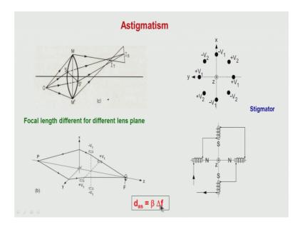
So, this is like that of a comma which you can see. This is that shape this aberration also has to be. So, these are all the two aberrations of the microscope and this is also related to the spherical aberration coefficient C s. What is the other aberration which arises in a microscope? This is called as the astigmatism that is if the lens itself is not perfectly spherical; the surface is not spherical here.
