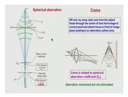
This aberration itself we have just shown it for a point object which is going there on the optic axis and we do not get point image, but it is an image which is spread out in space. If we consider it as waves which are emanating from the sample and then, propagating, then we can make out that the rays which are away from the optic axis, they are bent. The clusters have been bent a little bit more forward. Because of that only this sort of aberration which is occurring.
