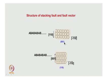
Now, we will come back to stacking fault. What is the stacking fault? In FCC let us take that case, it is the easiest one which has been very studied crystallographically as well as in microscopy also. What is the sort of a defect which it introduces, introduction of fault. What it does shifting of an atom layer, but what is the fault vector.
