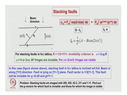
Now, suppose such a fault line is inclined like this. And the fault vector is always in these direction. Now you see that when the fault is inclined up to this it is a there is phase shift which will introduce because of right.
