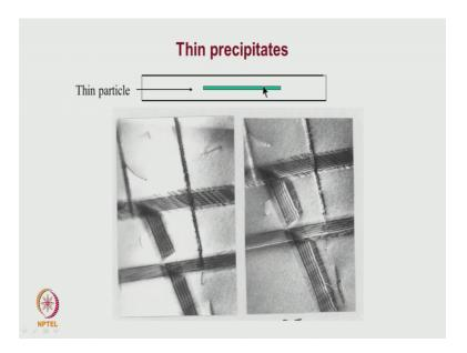
That precipitate, what it is does is that the beam which is enters here to a beam which comes down. It may introducing only a small phase shift. If such phase shift is introduced that will manifest itself as a fringe contrast, this is one case which comes from a precipitate here also you get a fringe contrast. So, there are various reasons why
