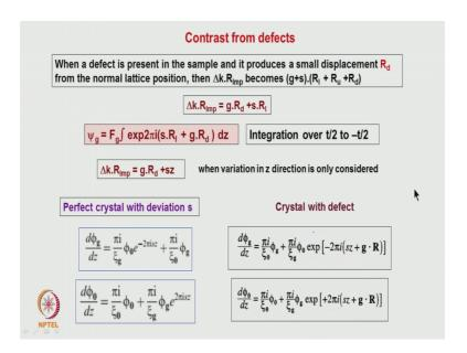
So, that is essentially governed by delta k dot R imp. Which represents the position of each atomic point in the unit cell. This value equals whether an integer or not, correct? When we substitute this value delta k equals g plus s and the defect itself can be written as position of each of the unit cell represented by a point which is called as R 1. Plus the position of atoms within the unit cell which is given by R u plus deviation defect is R d.
